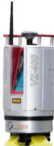
**Figura 3.2:** Escáner Riegl VZ-400.
