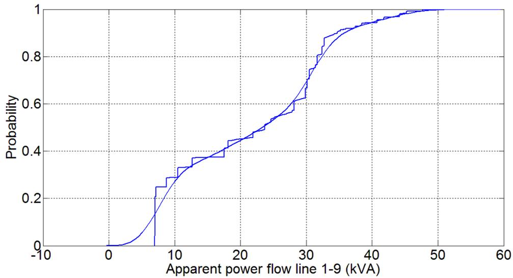
Figure 4.7: Cumulative distribution function for apparent power flow in line 1-9 Uncontrolled
