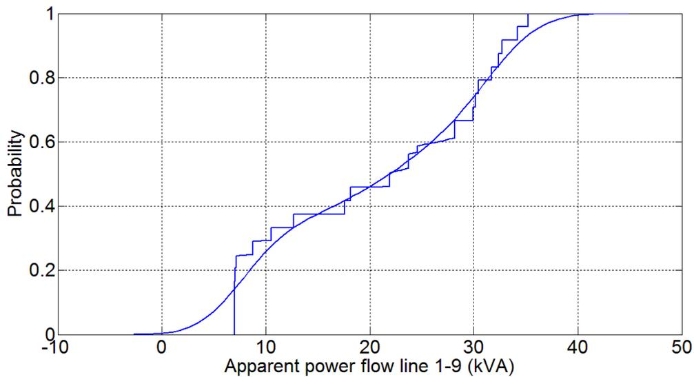
Figure 4.8: Cumulative distribution function for apparent power flow in line 1-9 Aggregator
