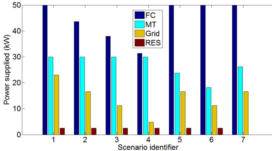
Figure 3.2: OPF correcting measures in power output
