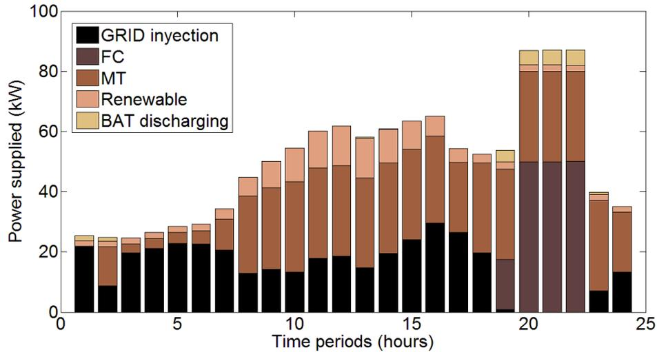
Figure 2.14: Microgrid power supply with DSM,  $k=12$
