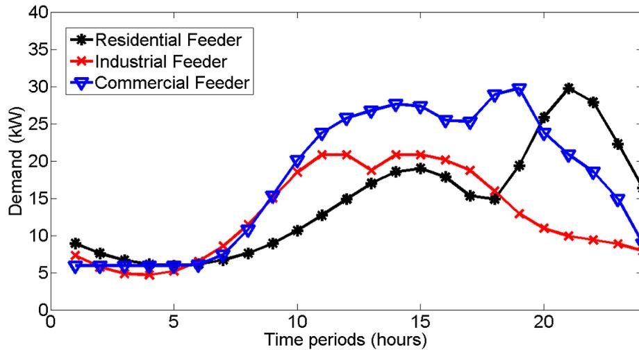
Figure 2.8: Electricity Loads in the MG Feeders
