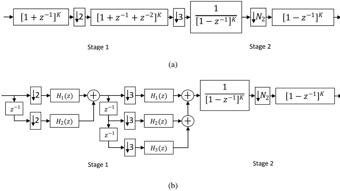
Fig. 4.10 Decimator structure (a) *Direct-3* and (b) *Polyphase-3*, for  $M=2 \cdot 3N_2$ .
