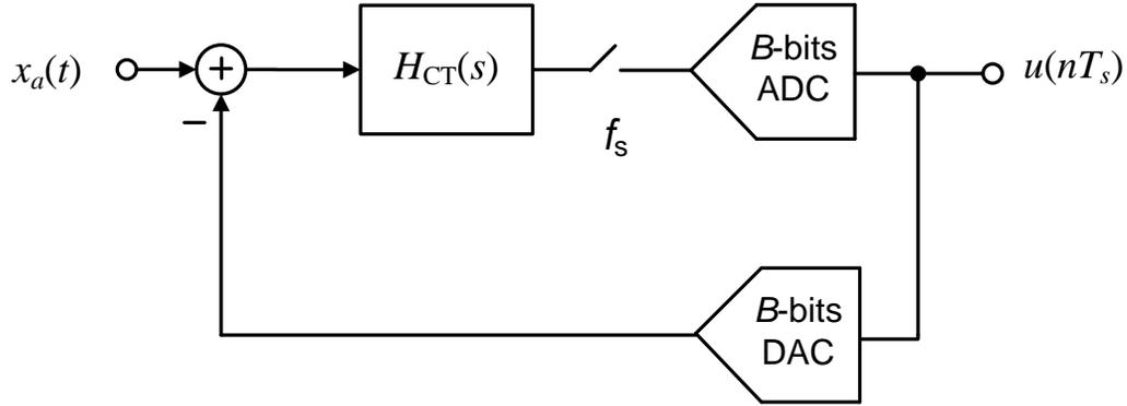
Fig. 1.8 Continuous-Time  $\Sigma\Delta$ M.
