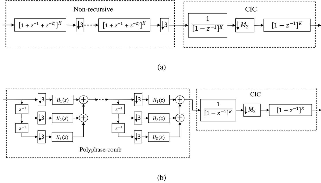
Fig. 4.17 Proposed structure for  $M=3^P$ : (a) *NR-CIC-1* and (b) *NR-CIC-2*.
