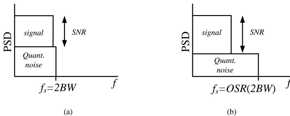
Fig. 1.4 Quantization noise power in (a) a Nyquist ADC and (b) an oversampled ADC.
