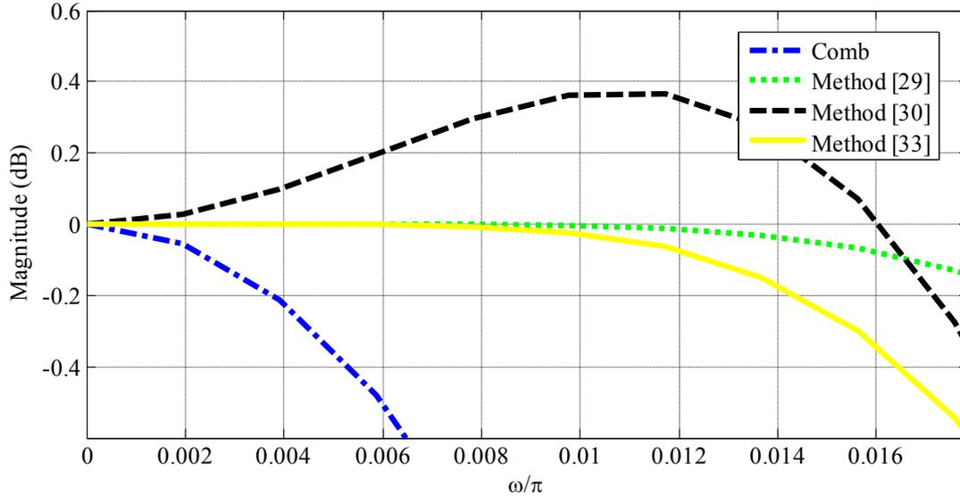
Fig. 2.3 Passband compensation in comb-based decimation filters.
