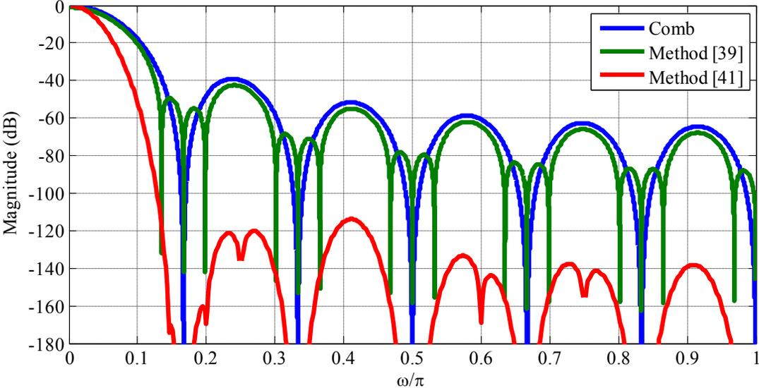
Fig. 2.4 Stop-band attenuation improvement.
