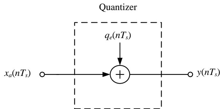
Fig. 1.3 Linear model of a quantizer.
