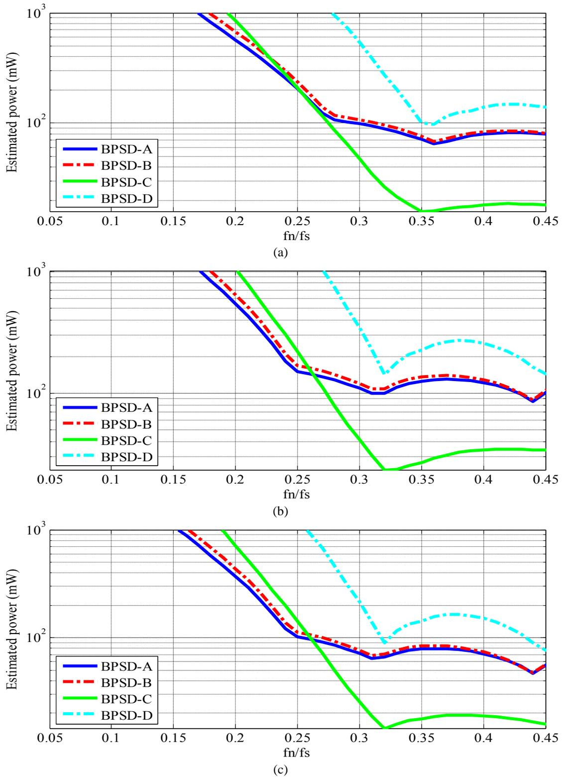
Fig. 3.18. Estimated power consumption versus  $f_n$  for: (a) RZ DAC, (b) NRZ DAC and (c) RCoS DAC.
