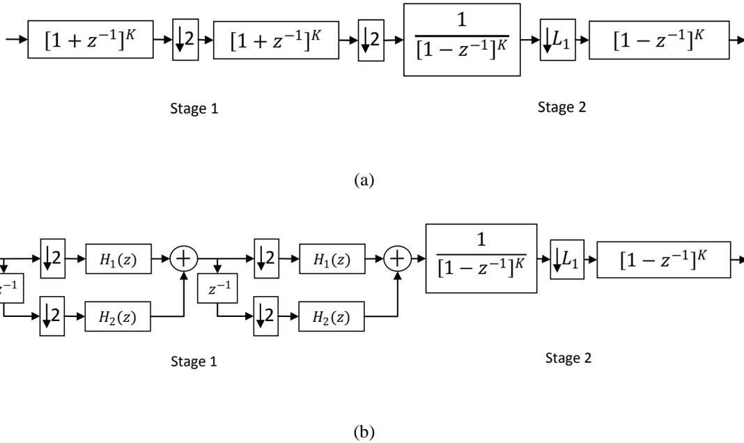
Fig. 4.6 Decimator structure (a) *Direct-1* and (b) *Polyphase-1*, for  $M=4L_1$ .
