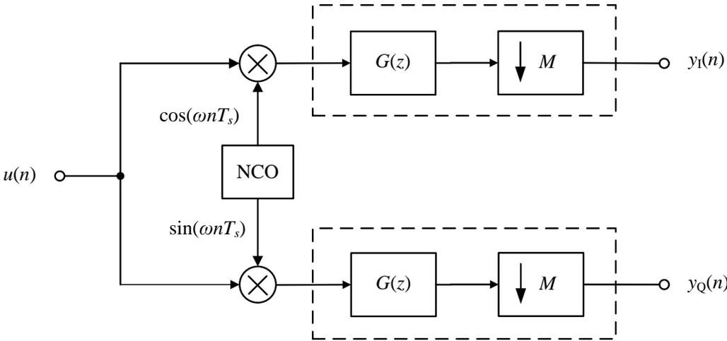
Fig. 1.16 Block diagram of a DDC.
