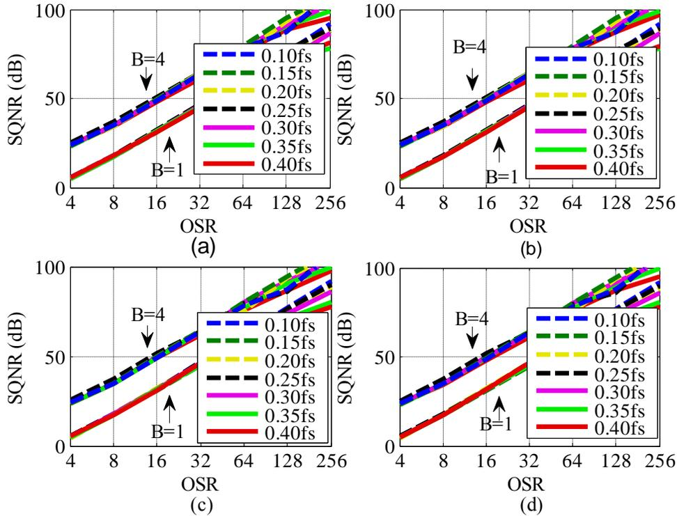
Fig. 3.11. SQNR versus OSR and  $B$  for different cases of  $f_n$ . (a)  $\text{BP}\Sigma\Delta\text{-A}$ . (b)  $\text{BP}\Sigma\Delta\text{-B}$ . (c)  $\text{BP}\Sigma\Delta\text{-C}$ . (d)  $\text{BP}\Sigma\Delta\text{-D}$ .
