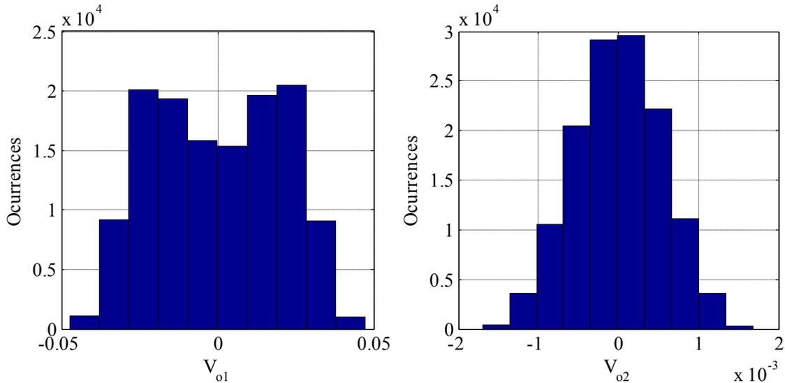
Fig. 3.26. Histograms of the resonator outputs considering  $B = 1$  and  $f_n = f_s / 4$  for the BP CT- $\Sigma\Delta$ M shown in Fig. 3.25(c): (a) Front-end resonator output,  $v_{o1}$ . (b) Back-end resonator output,  $v_{o2}$ . (1-V full-scale reference voltage).
