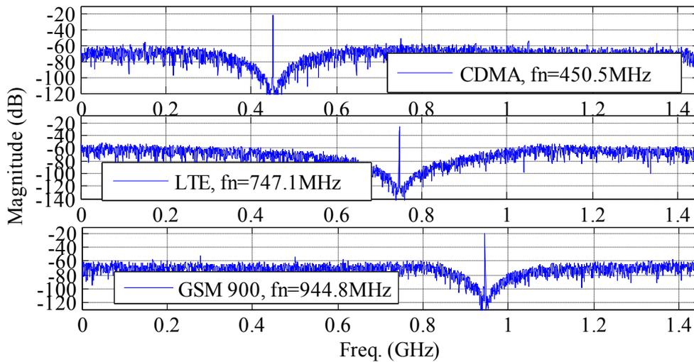
Fig. 3.19. Output spectra computed from Cadence-Spectre® macromodel simulations of BP $\Sigma\Delta\text{-B}$  with NRZ DAC,  $B = 4$  and  $f_s = 3\text{GHz}$ .
