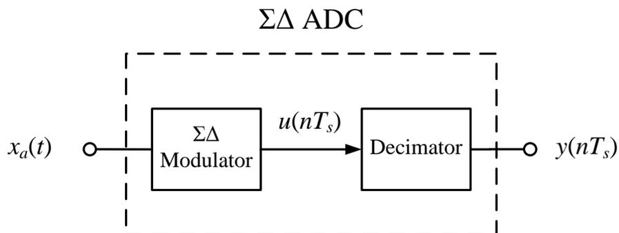
Fig. 1.5  $\Sigma\Delta$  ADC: Modulator and Decimator.
