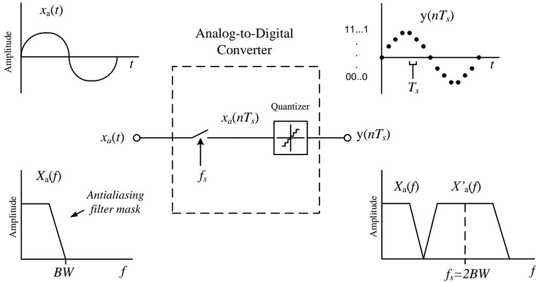
Fig. 1.1 Analog-to-Digital conversion.
