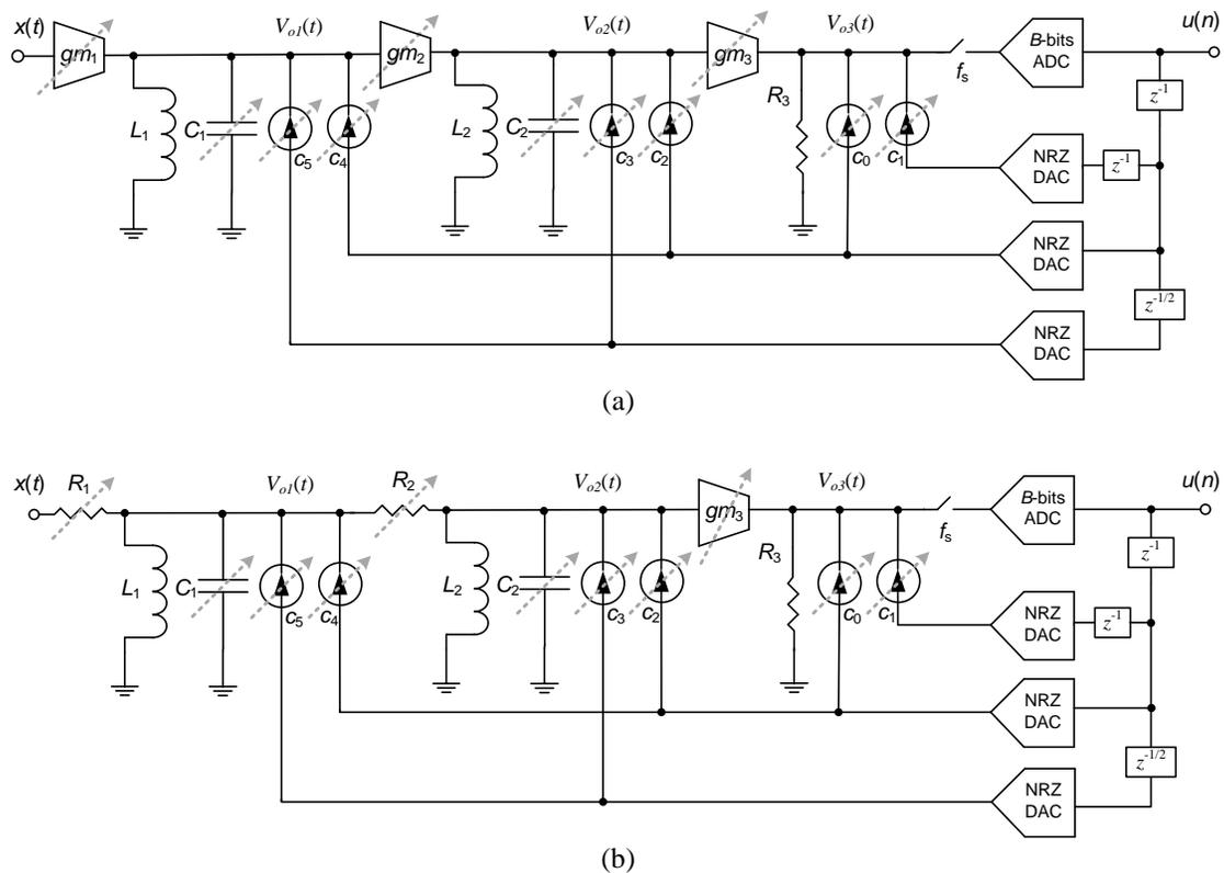
Fig. 3.23. Conceptual circuit implementation of the BP CT- $\Sigma\Delta$ M in Fig. 3.8(a) considering: (a) Active loop-filter. (b) Passive loop-filter. (Dashed arrows indicate that the circuit elements are programmable.)
