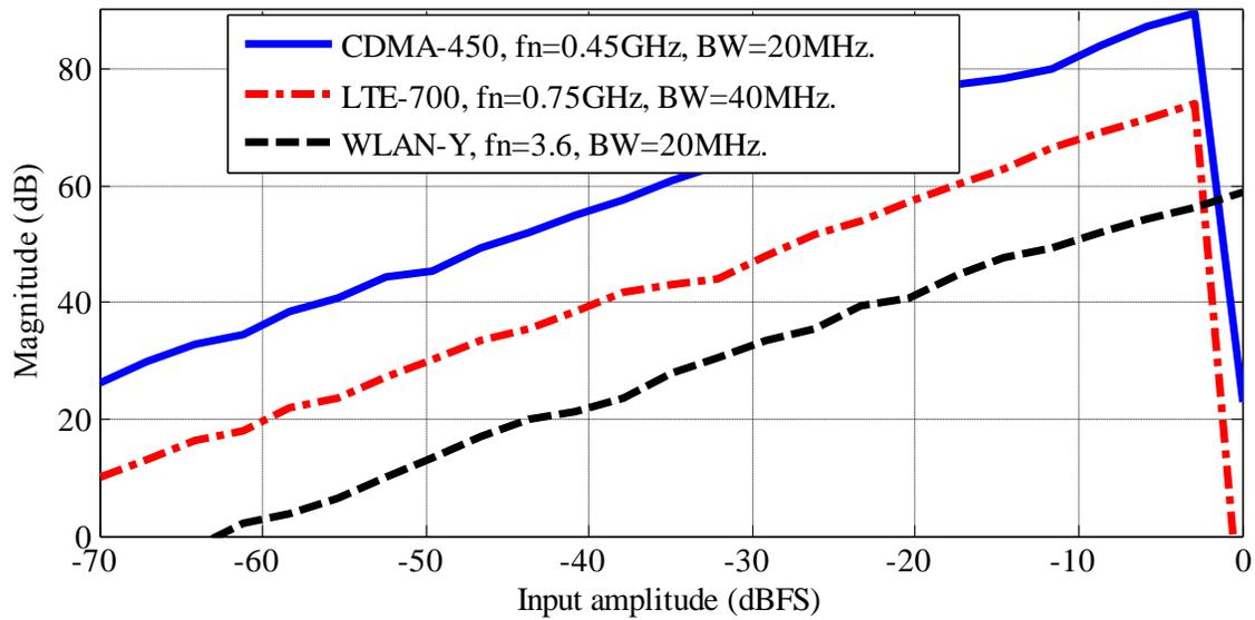
Fig. 3.22. SNR vs. input amplitude for different standards and  $f_s = 2\text{GHz}$ .
