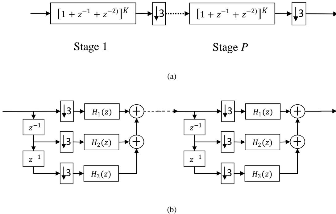
Fig. 4.15 Non-recursive comb for  $M = 3^P$ : (a) direct form implementation and (b) polyphase form implementation.
