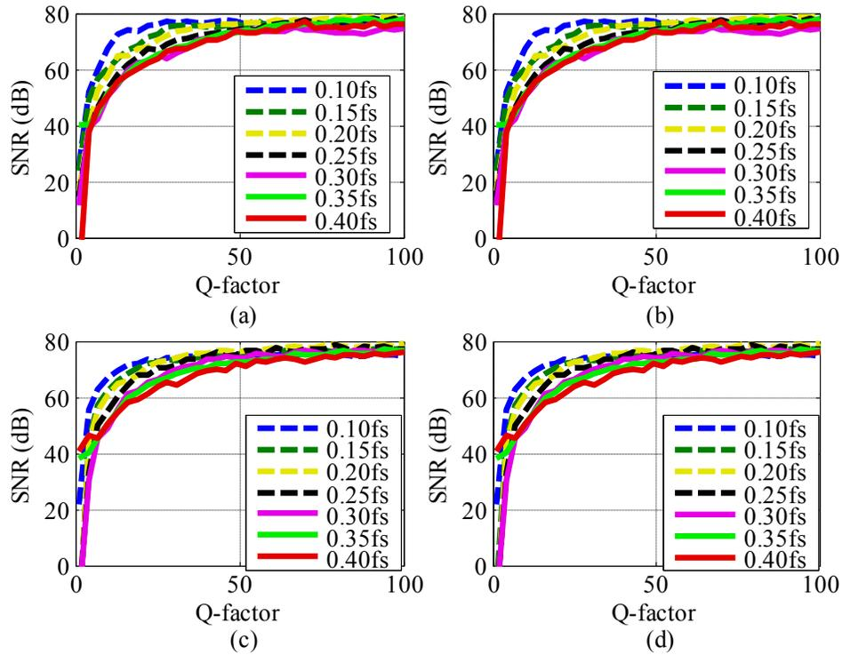
Fig. 3.15. Effect of the finite quality factor on the SNR with RZ DAC and  $B = 4$  for: (a)  $\text{BP}\Sigma\Delta\text{-A}$ , (b)  $\text{BP}\Sigma\Delta\text{-B}$ , (c)  $\text{BP}\Sigma\Delta\text{-C}$  and (d)  $\text{BP}\Sigma\Delta\text{-D}$ .
