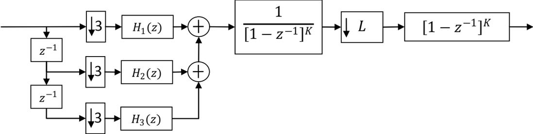
Fig. 4.20 Polyphase-4 structure, for decimation factors that are multiples of three.
