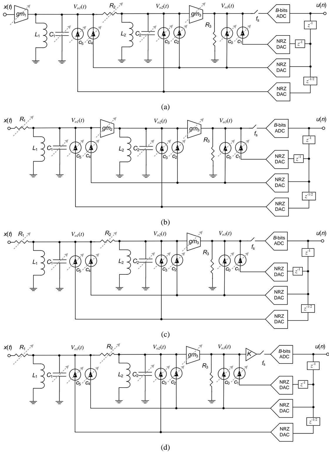
Fig. 3.25. Conceptual schematics of the proposed BP CT- $\Sigma\Delta$ Ms considering: (a) An active front-end resonator and a passive second resonator. (b) A passive front-end resonator and an active second resonator. (c) Both passive resonators with active gain at the summation. (d) A fully passive feed-forward filter.
