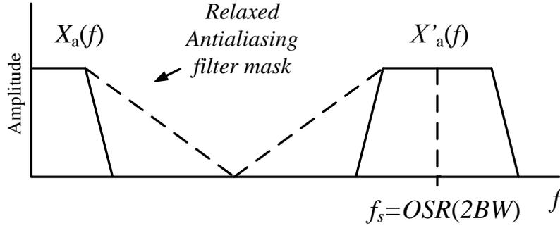
Fig. 1.2 Oversampling and relaxed antialiasing filter mask.
