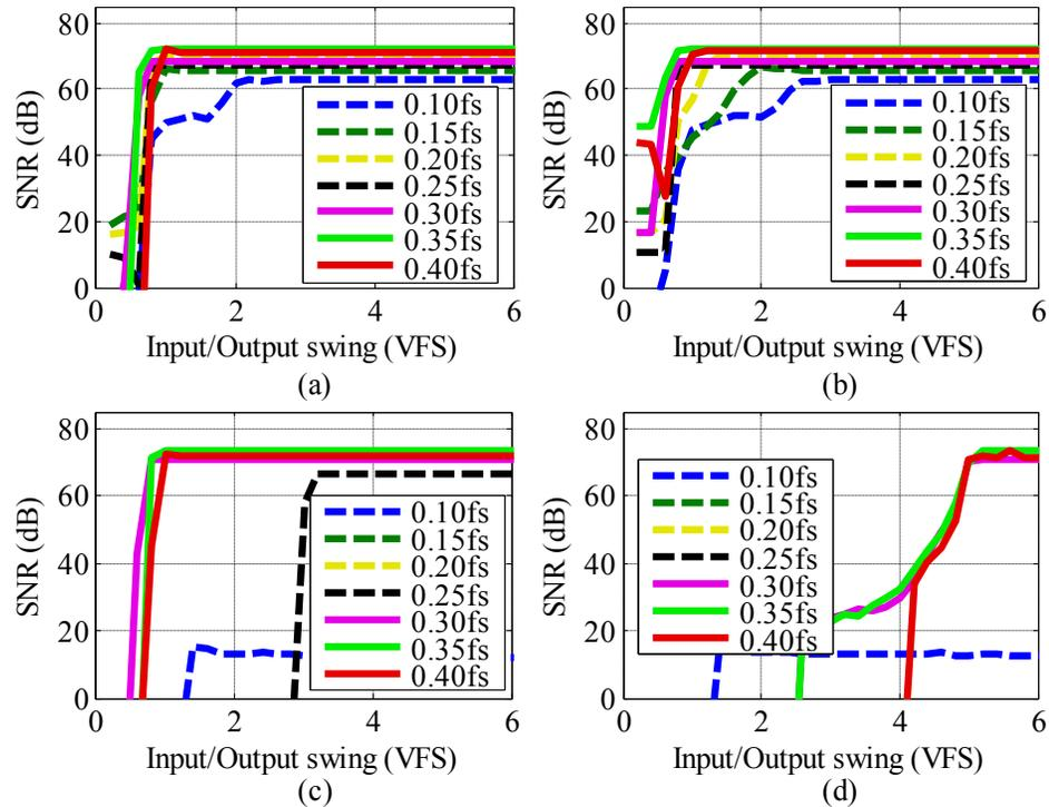
Fig. 3.14. Effect of I/O the SNR with RCoS DAC and  $B = 4$  for: (a)  $\text{BP}\Sigma\Delta\text{-A}$ , (b)  $\text{BP}\Sigma\Delta\text{-B}$ , (c)  $\text{BP}\Sigma\Delta\text{-C}$  and (d)  $\text{BP}\Sigma\Delta\text{-D}$ . (Note that the behavior of  $\text{BP}\Sigma\Delta\text{-C}$  and  $\text{BP}\Sigma\Delta\text{-D}$  becomes unstable for  $f_n/f_s = 0.1$ ).
