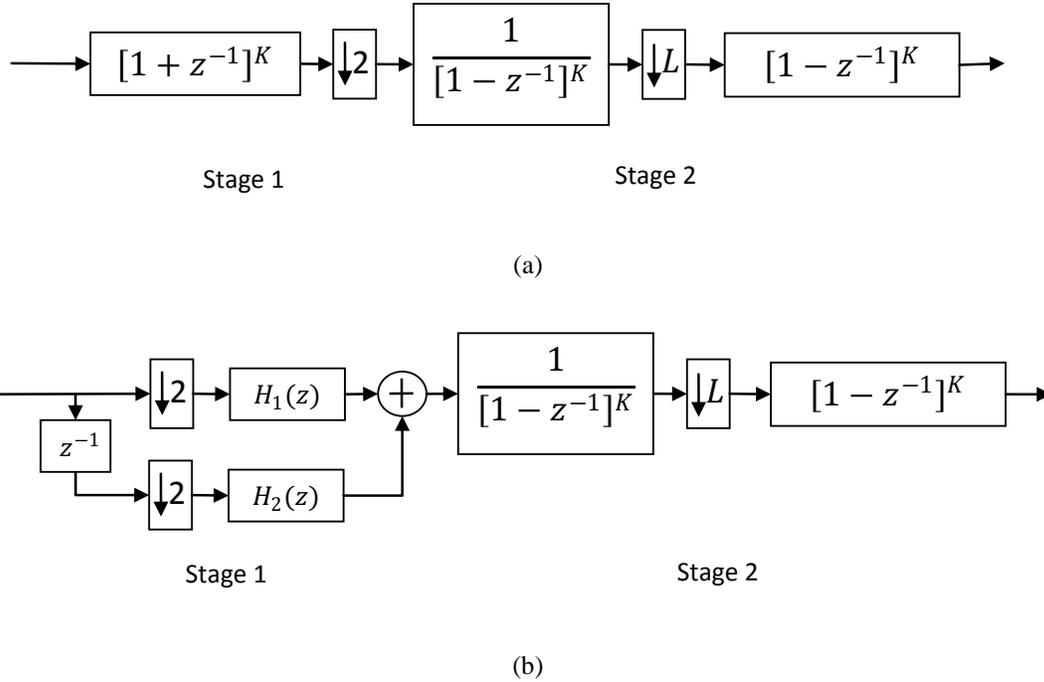
Fig. 4.8 Decimator structure (a) *Direct-2* and (b) *Polyphase-2*, for  $M=2L$ .
