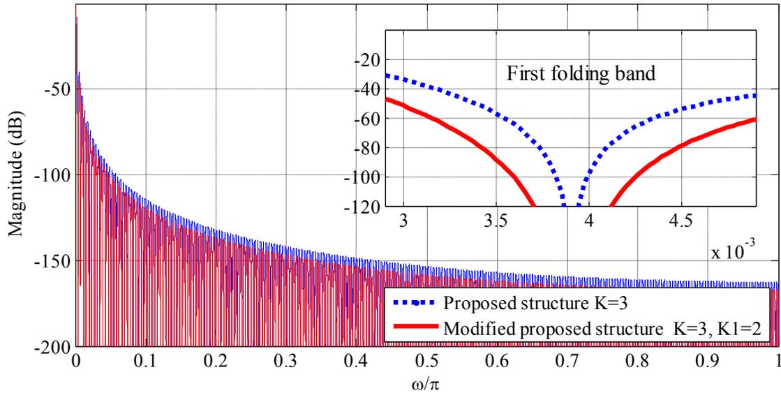
Fig. 4.5 Magnitude response for proposed and modified proposed structure,  $M=512$ .
