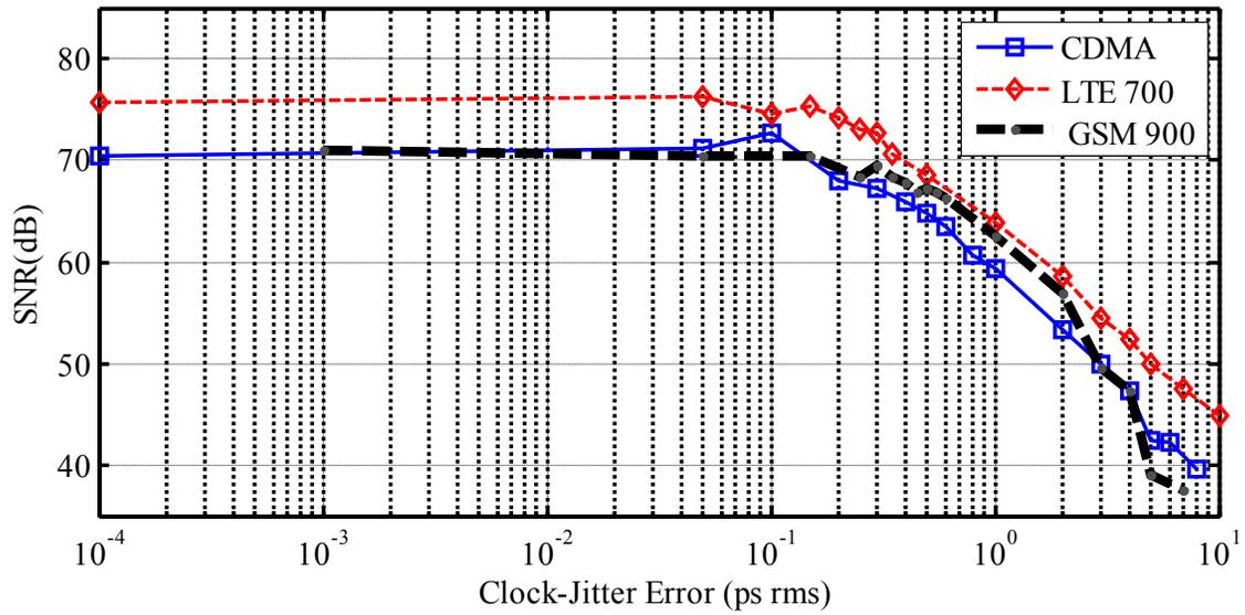
Fig. 3.21. SNR vs. clock-jitter error for different standards.
