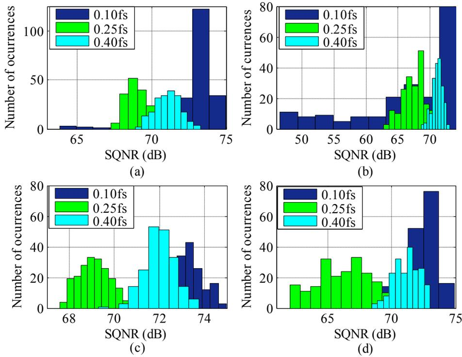
Fig. 3.17. Monte Carlo simulation with NRZ DAC and  $B = 4$ : (a)  $\text{BP}\Sigma\Delta\text{-A}$ ,  $\sigma = 1\%$ , (b)  $\text{BP}\Sigma\Delta\text{-A}$ ,  $\sigma = 2.5\%$ , (c)  $\text{BP}\Sigma\Delta\text{-B}$ ,  $\sigma = 1\%$ , (d)  $\text{BP}\Sigma\Delta\text{-B}$ ,  $\sigma = 2.5\%$ .
