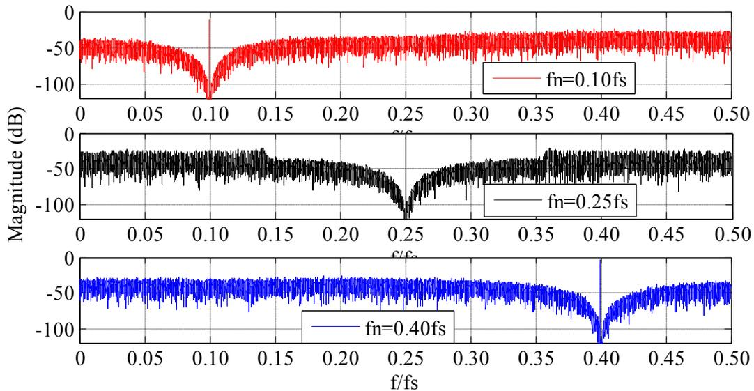
Fig. 3.2. Output spectra of modulator in Fig. 3.1 for different values of  $f_n$ . (Note that the *idle tones* observed for  $f_n = f_s/4$  are due to the correlation between the quantization error and the input signal, which is reduced in practice by nonidealities and/or using multi-bit quantization).
