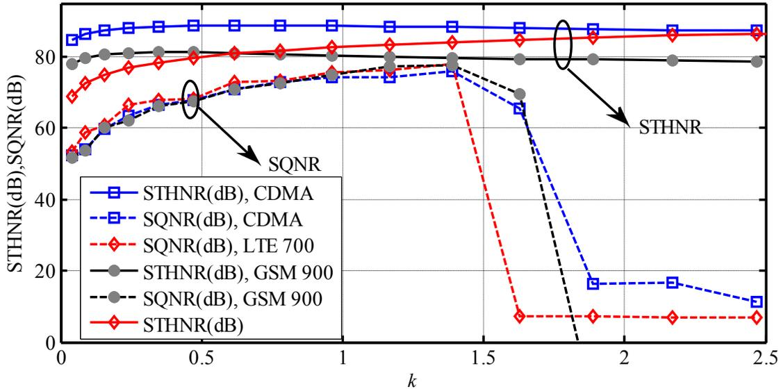
Fig. 3.20. Effect of tuning  $k$  on SQNR and STHNR for different standards.
