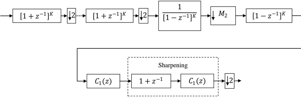
Fig. 4.25 *Corrected-2* structure.
