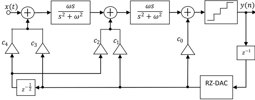
Fig. 3.1. Block diagram of a fourth-order LC-based BP CT- $\Sigma\Delta$ <sup>1</sup>.
