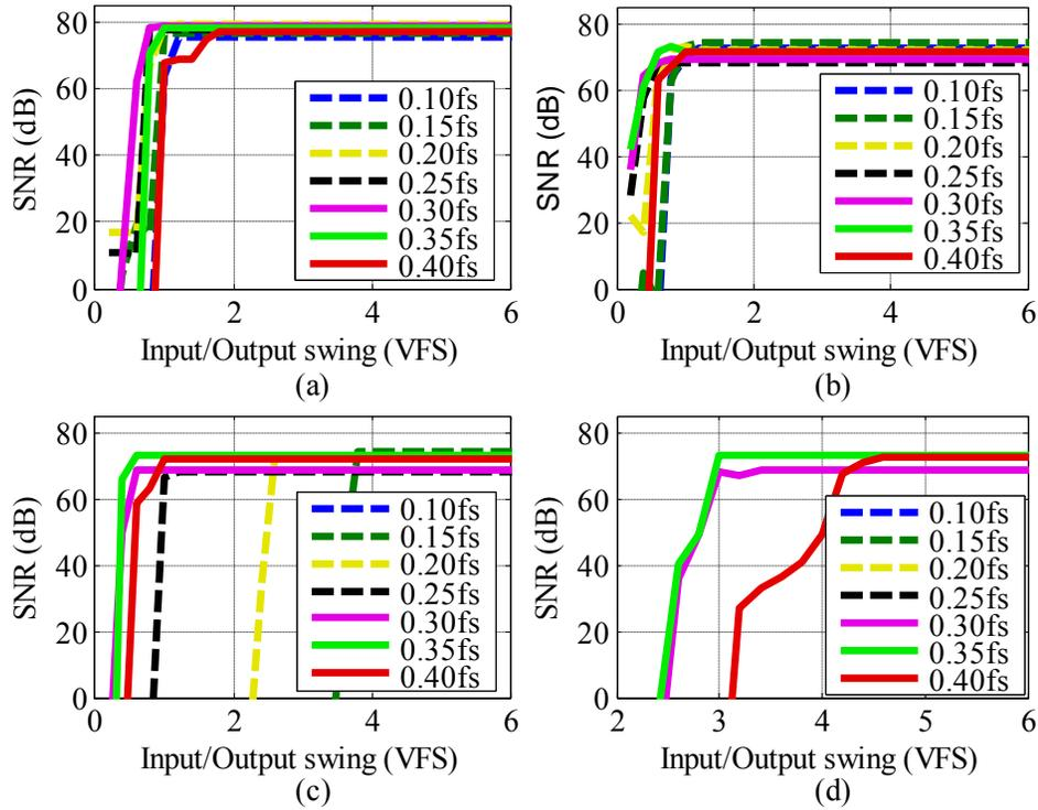
Fig. 3.13. Effect of I/O the SNR with NRZ DAC and  $B = 4$  for: (a)  $\text{BP}\Sigma\Delta\text{-A}$ , (b)  $\text{BP}\Sigma\Delta\text{-B}$ , (c)  $\text{BP}\Sigma\Delta\text{-C}$  and (d)  $\text{BP}\Sigma\Delta\text{-D}$ .
