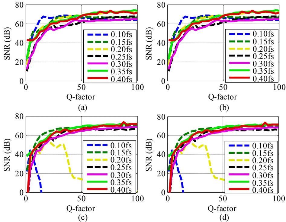
Fig. 3.16. Effect of the finite quality factor on the SNR with RCoS DAC and  $B = 4$  for: (a)  $\text{BP}\Sigma\Delta\text{-A}$ , (b)  $\text{BP}\Sigma\Delta\text{-B}$ , (c)  $\text{BP}\Sigma\Delta\text{-C}$  and (d)  $\text{BP}\Sigma\Delta\text{-D}$ .
