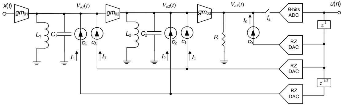
Fig. 3.10. Conceptual Gm-LC schematic of the BP CT- $\Sigma\Delta$ M in Fig. 3.1.
