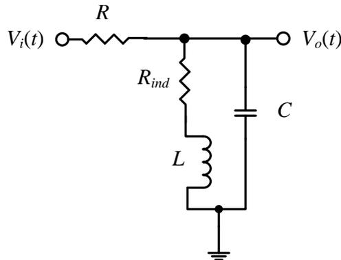
Fig. 3.28. Equivalent circuit used to model a passive resonator with a parasitic series resistance,  $R_{ind}$ .
