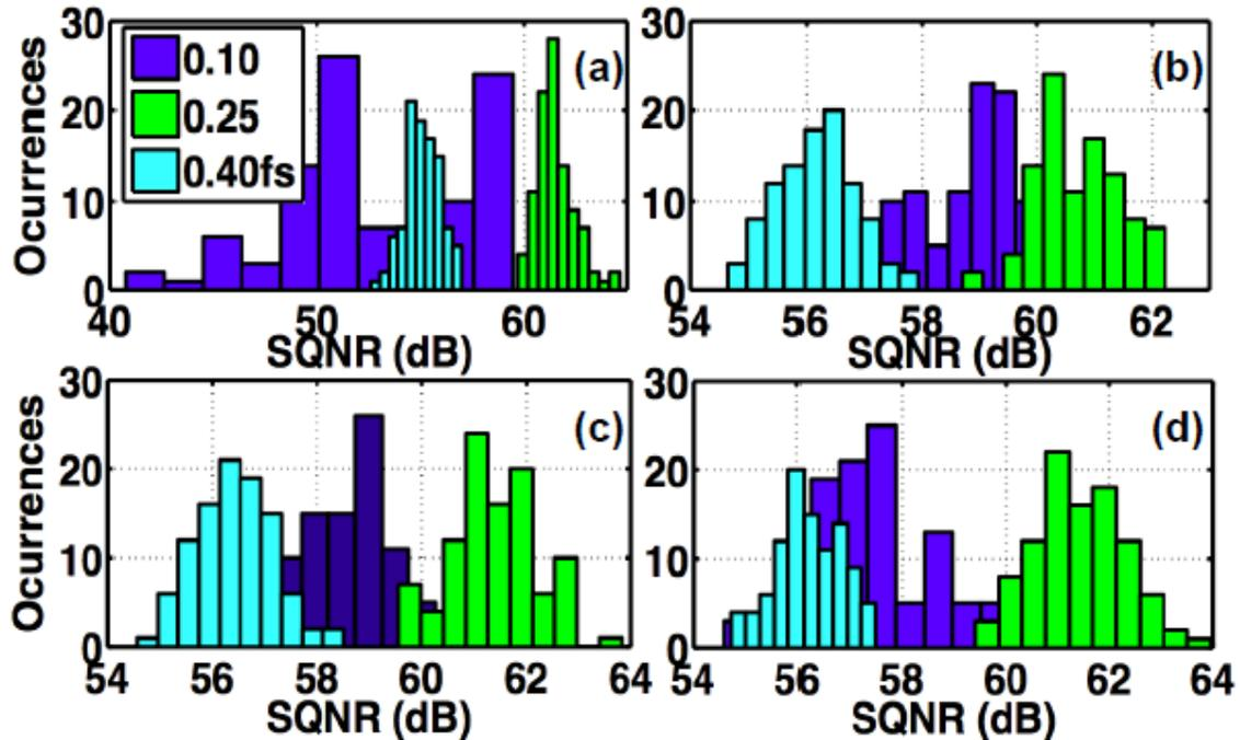
Fig. 3.30. Monte Carlo simulation of the BP CT- $\Sigma\Delta$ Ms under study with  $\sigma = 2\%$ , OSR=50: (a) Hybrid-1, (b) Hybrid-2, (c) Passive-1, (d) Passive-2.
