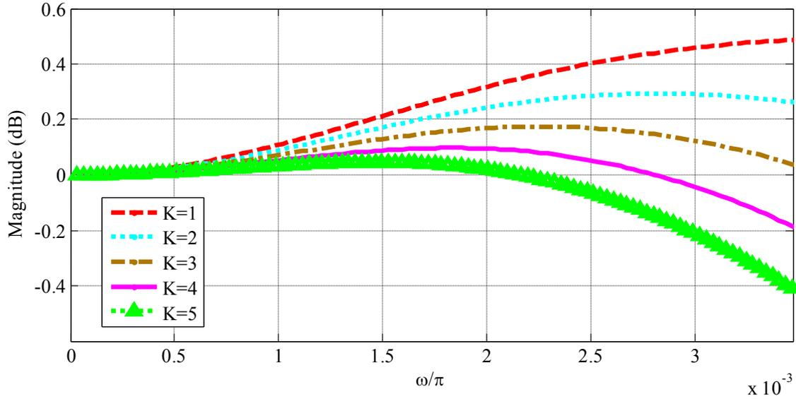
Fig. 4.27. Magnitude response in the passband of corrected-2 structure, considering different values of  $K$ .
