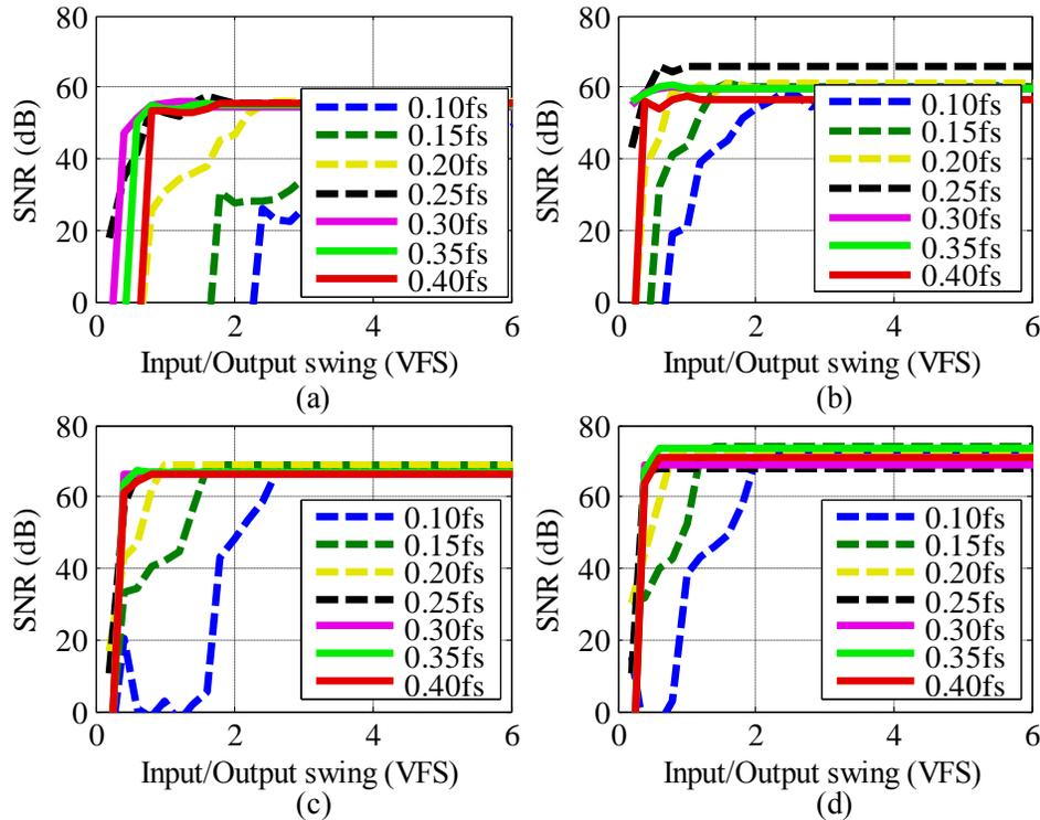
Fig. 3.12. Effect of I/OS (relative to VFS) on the SNR of BP $\Sigma\Delta$ -A with RZ DAC and (a)  $B = 1$ , (b)  $B = 2$ , (c)  $B = 3$  and (d)  $B = 4$ .
