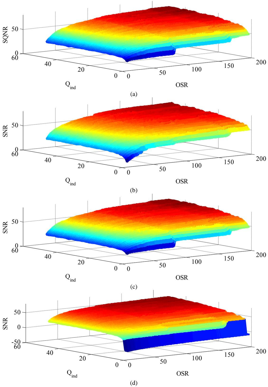
Fig. 3.29. Impact of  $Q_{ind}$  on the SNR for the BP CT- $\Sigma\Delta$ Ms of Fig. 25: (a) Hybrid-1, (b) Hybrid-2, (c) Passive-1, (d) Passive-2.
