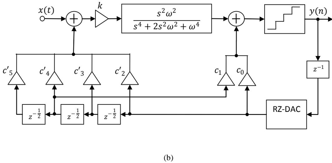
Fig. 3.7. Alternative implementations of BP CT- $\Sigma\Delta$ M based on a single section LC loop filter. (a) With a single preamplification factor (denoted as BP $\Sigma\Delta$ -C). (b) With a preamplification distributed between the feedforward and the feedback blocks in the modulator chain (denoted as BP $\Sigma\Delta$ -D).
