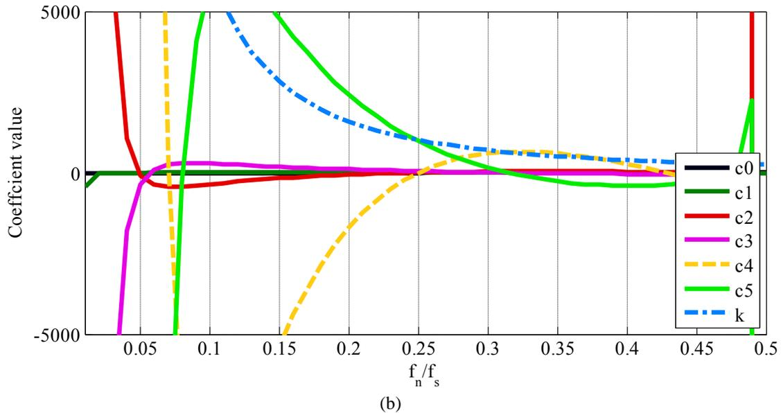
Fig. 3.24. Loop-filter coefficients,  $c_i$ , versus  $f_n = f_s$  for: (a) the active modulator and (b) the passive versions of the BP CT- $\Sigma\Delta\text{M}$  shown in Fig. 3.23.
