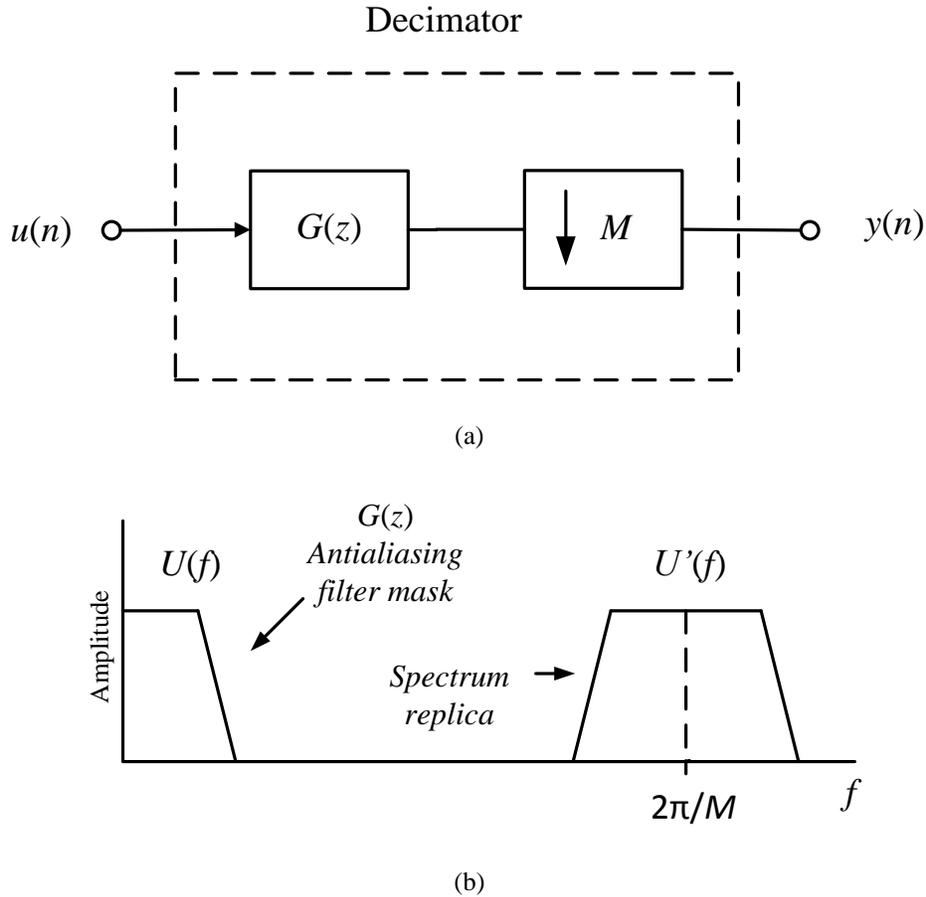
Fig. 1.11 (a) Decimator or decimation filter, and (b) downsampling in the frequency domain.
