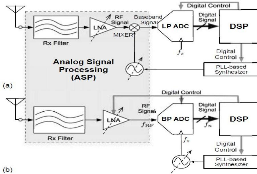
Fig. 2.1 Conceptual SDR receiver based on a: (a) LP ADC. (b) BP ADC.
