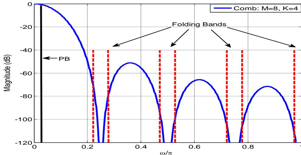
Fig. 1.13 Magnitude response of a comb filter with  $M=8$  and  $K=4$ .
