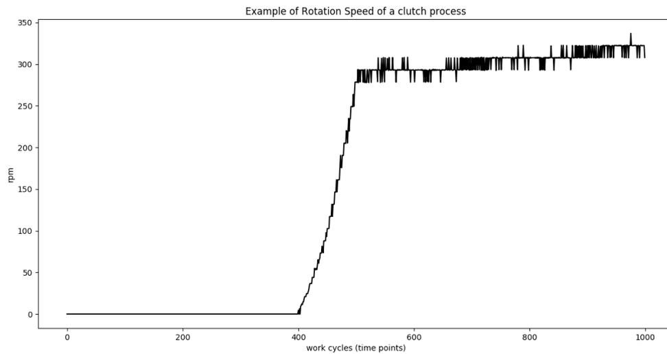
**Figure 5.2:** Example of Rotation Speed signal of Press-Machine case study for a clutch simulation.
