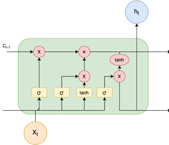
**Figure 2.9:** Representation of a LSTM block with its components [4].
