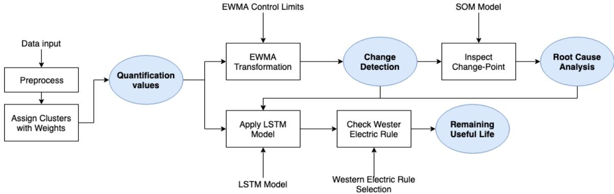
**Figure 4.6:** Test Methodology of the Predictive Maintenance workflow with the ReWAOI algorithm.
