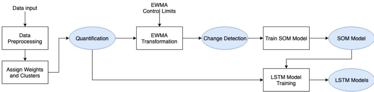
**Figure 4.3:** Part III of the Train Methodology of the Predictive Maintenance workflow with the ReWAOI algorithm.
