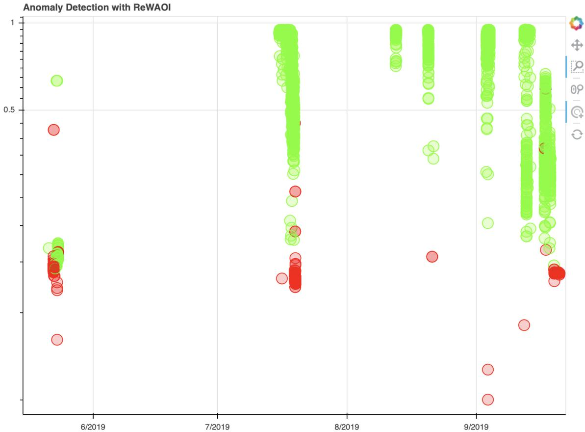
**Figure 6.13:** Anomaly Detection performed by ReWAOI algorithm. Green points refer to correct executions, and red points to anomalies.
