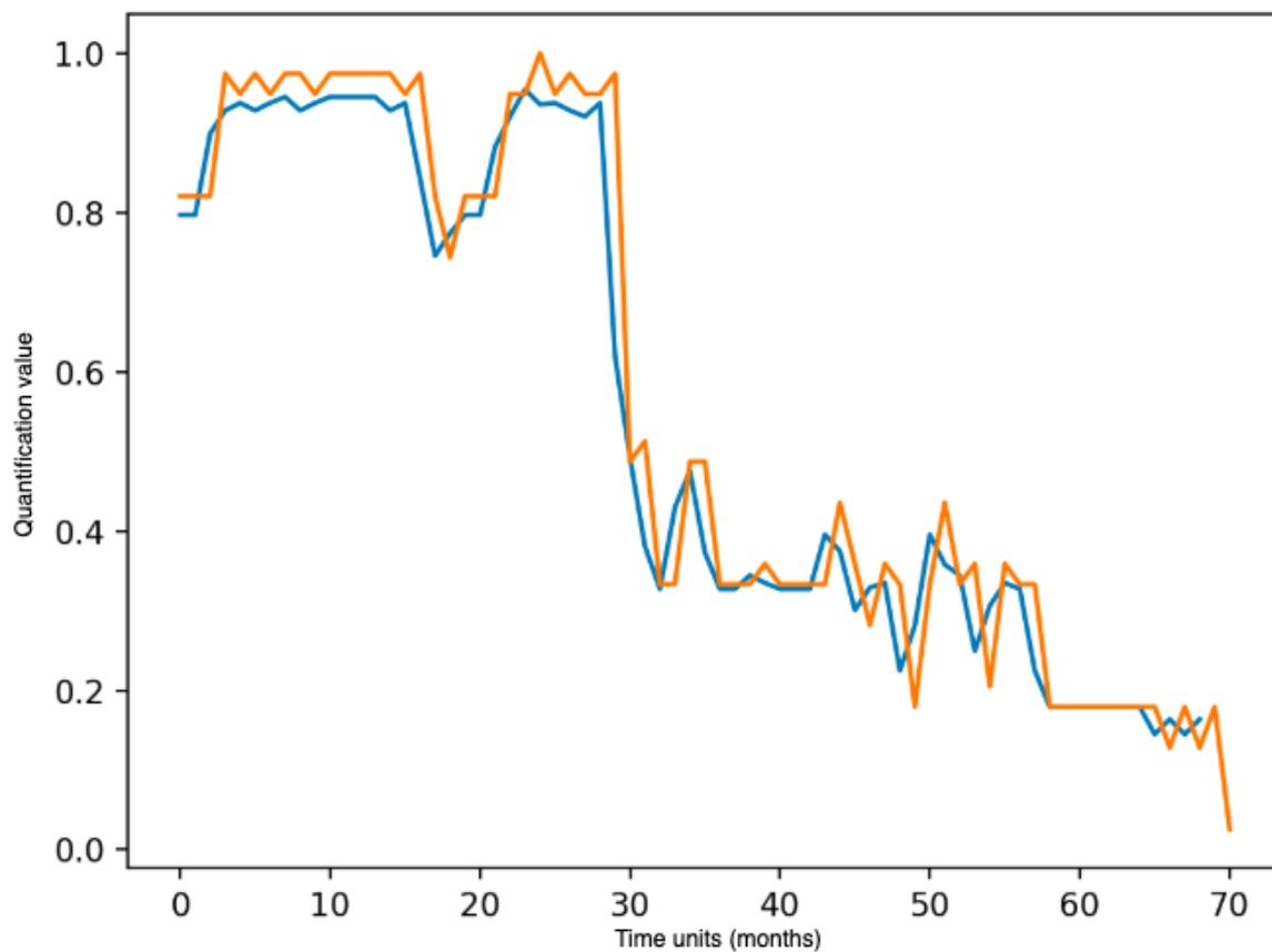
**Figure 6.2:** Remaining Useful Life prediction performed by an AR model in the Press-Machine case study.
