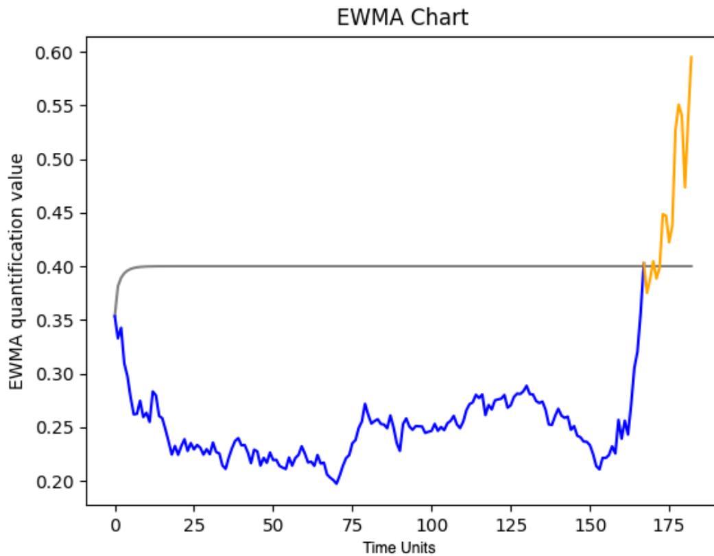
**Figure 6.5:** Example of representation of a simulation in an EWMA control chart.
