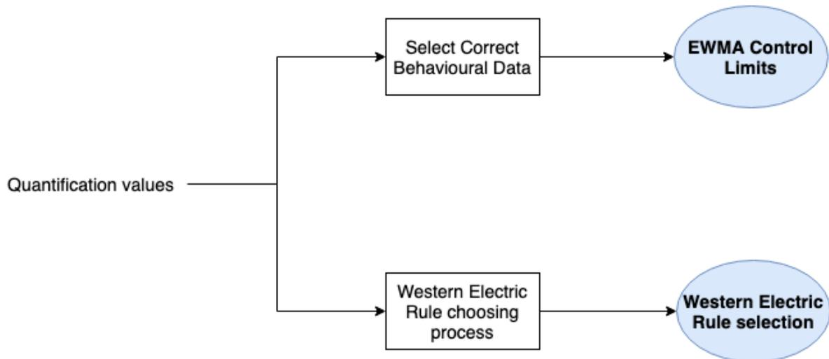
**Figure 4.2:** Part II of the Training Phase of the Predictive Maintenance workflow with the ReWAOI algorithm.
