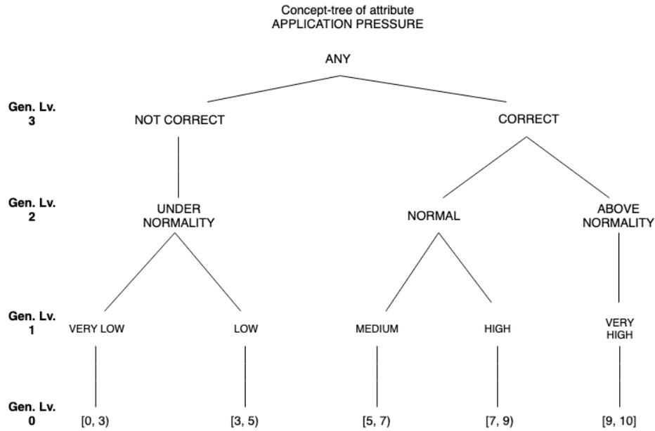
**Figure 3.2:** Example of a concept-tree or concept-hierarchy of a Predictive Maintenance attribute: Application Pressure.
