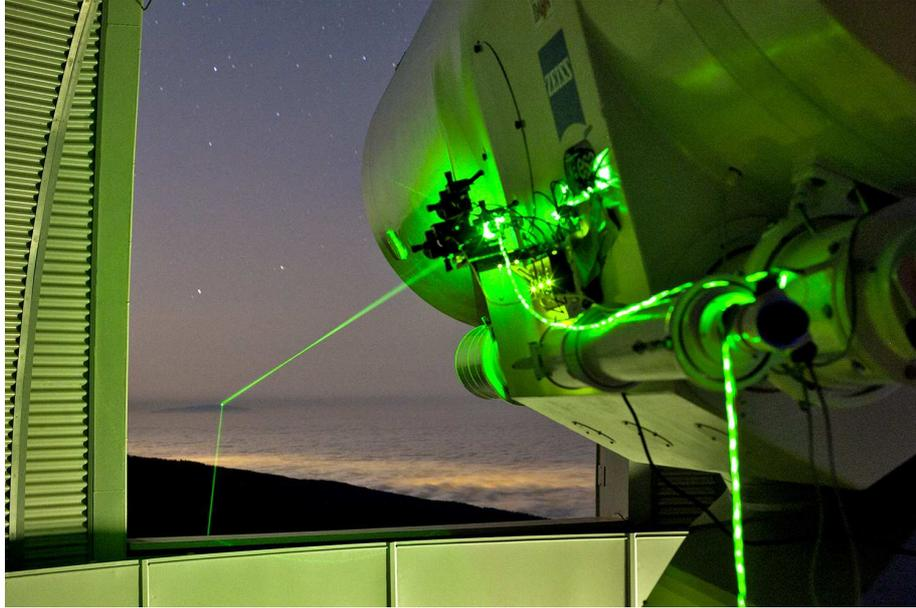
Figure 4.1: Image of the OGS telescope, located at Izaña Observatory, Tenerife, laser connected with Roque de los Muchachos Observatory in the island of La Palma.
