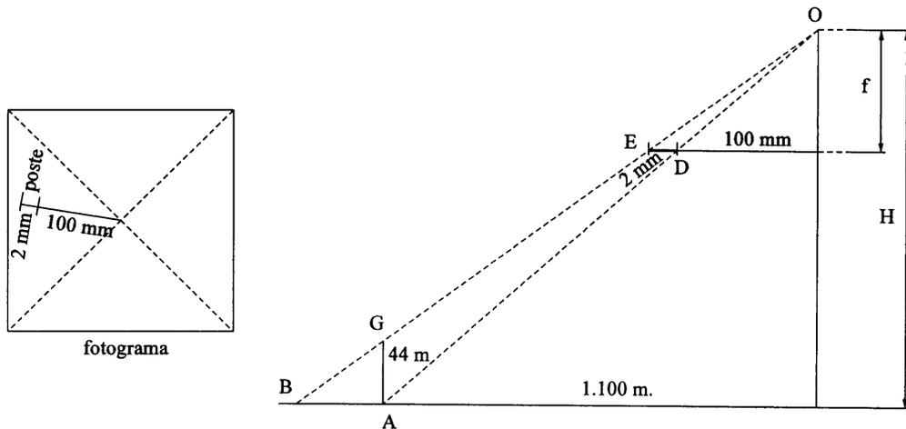
$$E = \frac{1}{e} = \frac{100\text{mm}}{1.100\text{m}} = \frac{0,1}{1.100} = \frac{1}{11.000} \quad E = \frac{1}{11.000} \quad \text{escala del fotograma}$$
