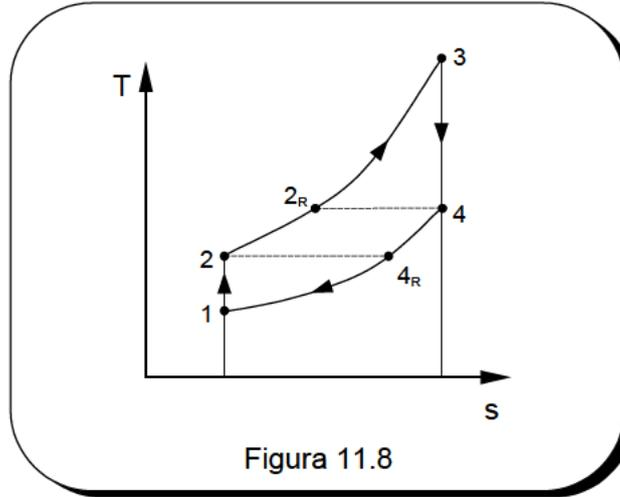
$$w_T = h_3 - h_4 = c_p(T_3 - T_4) = c_p(T_3 - T_{2R}) = q$$
