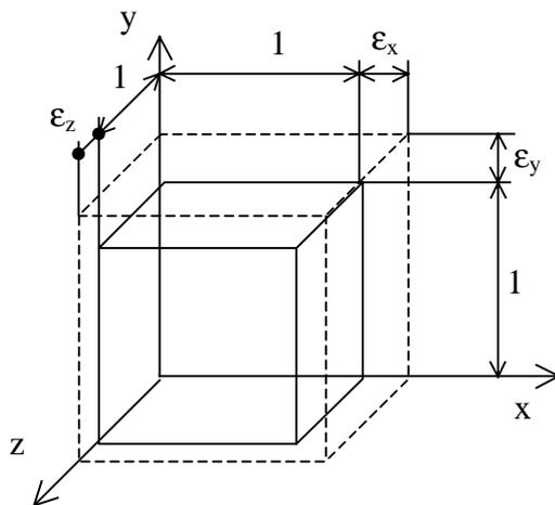
Figura 15.6 Deformaciones  $\epsilon_x$ ,  $\epsilon_y$ ,  $\epsilon_z$ **Ley de Hooke para tensión plana:**
