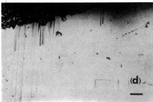
Fig.4.-Growth pyramids generated from: a) Microfractures and grain boundaries. b) Dissolution traces. c) Impurities. d) Edge. Scale bar 0.25 mm.
