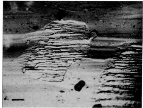
Fig.6.- Dauphiné twin domain and microdomain. The arrow indicates the teeth shaped edges. Scale bar 0.15 mm.
