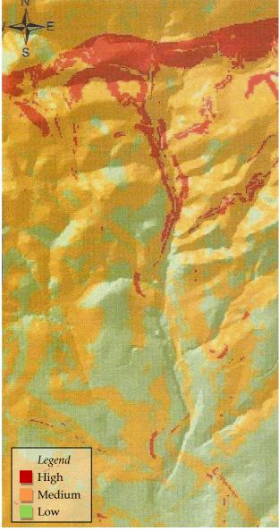
Fig. 3. Landslides Hazard Map through Digital Method
