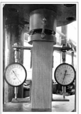
Figure 1 - Specimen tested in compression.
