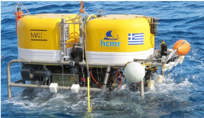
Fig 2. Recovering the ROV Max Rover (HCMR, Greece).
