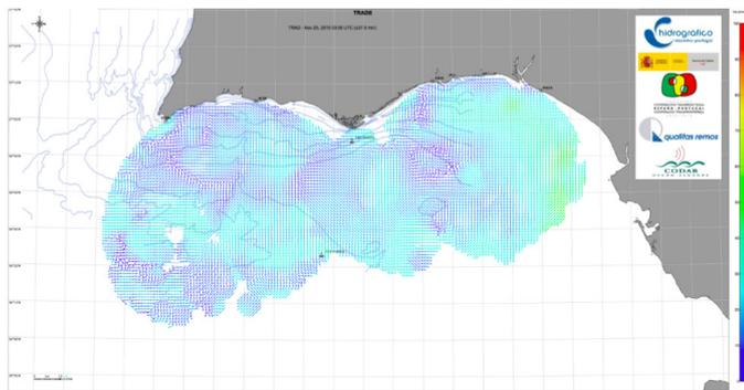
**Fig. 5 Algarve and Gulf of Cadiz HF Radar network with 4 x 13.5 MHz SeaSonde stations including the Sagres site. (Operated by the Instituto Hidrográfico of Portugal and Puertos del Estado of Spain, TRADE). Toscana, SICOMAR, Italia.**
