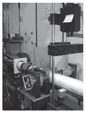
Figure 1: Multi-Sensor Core Logger of the Oregon State University, installed onboard the R/V Roger Revelle, showing the Gamma-Ray, electrical resistivity and Magnetic Susceptibility sensors. Also, a visible-image camera-scan device is shown.
