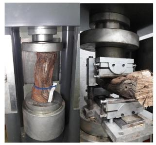
Fig. 2: A) Compression test of grapevine wood trunks; B) Flexural test of grapevine wood branches.
