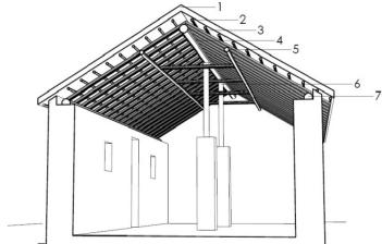
The pillars consist of wooden posts driven into the ground and reinforced by a brickwork sleeve to the same height as the load-bearing walls. These components in turn served as support when a second floor loft was built in later styles. The main beam would therefore rest on four supports, the two pillars or thicker side walls and the twin support posts (*pontones*). The process was completed by placing supporting collar ties (*tijeras*) in the higher areas.
