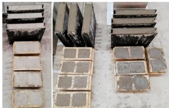
Figure 3. Curing of mortar samples (0.30 m × 0.30 m × 0.05 m).
