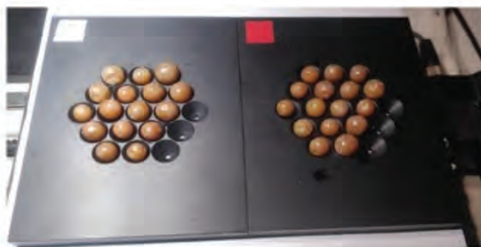
Figure 2. Fruit holders with the first subsample of 32 berries, 16 on each plate, prior HSI.
