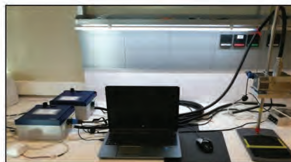
Figure 1. NIR spectrometer covering the range 1100–2100 nm.
