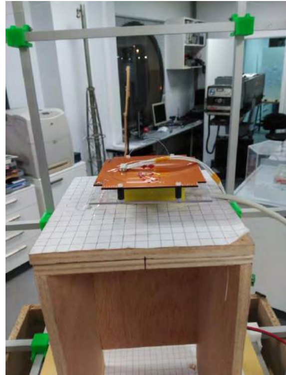
Fig. 12. Magnetometer and 1U magnetorquer inside the Helmholtz Cage
