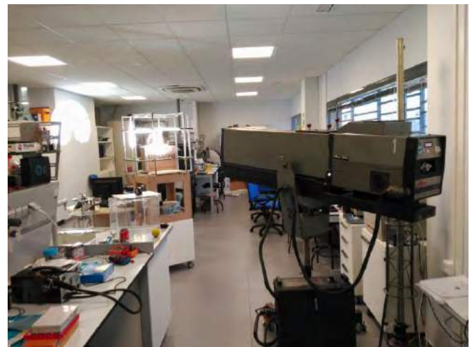
Fig. 16. Sun simulator illuminating a magnetorquer in the Helmholtz Cage
