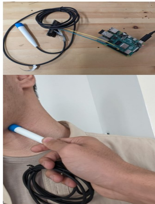
Figure 5. Type of connection of the CW sensor to the raspberry pi 4 and diagnosis of the carotid artery
