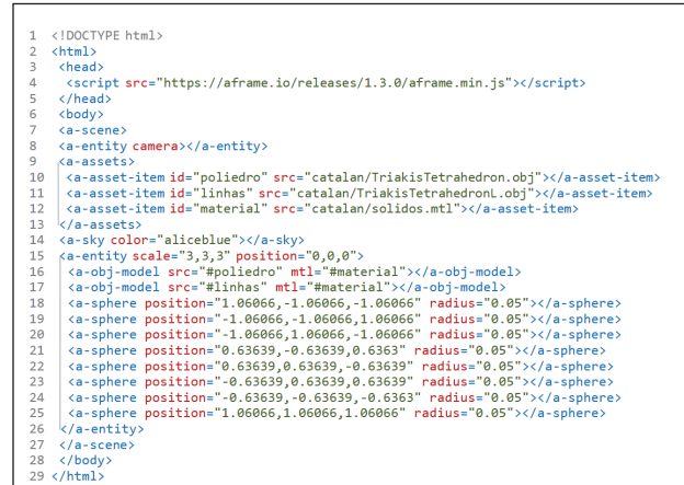
Figure 4: Code for modeling a Triakis Tetrahedron in VR using A-Frame resources.
