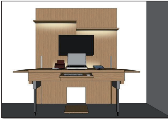
Figure 9: Multifunctional table with panel, open side flaps and keyboard, notebook and tablet supports.
