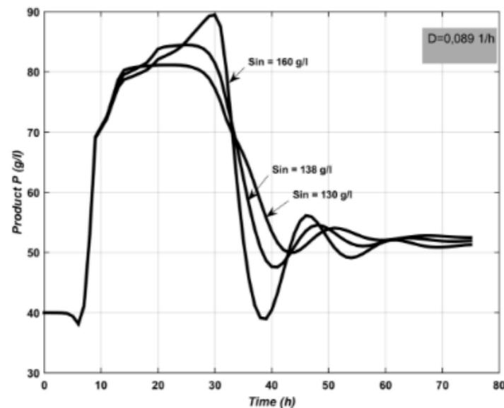
Fig. 3. Open-loop response to variations in initial substrate concentration.
