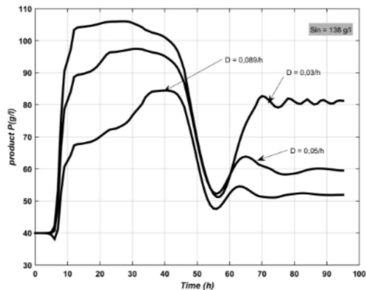
Fig. 2. Response of the open-loop reactor for different values of the Dilution Rate  $D$ .
