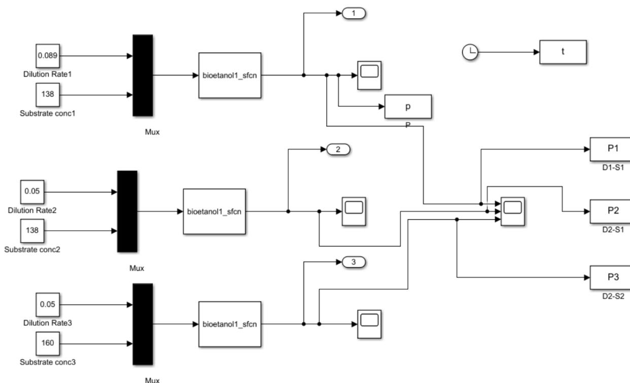
Fig. 1. Simulink diagram of the bioethanol production process.
