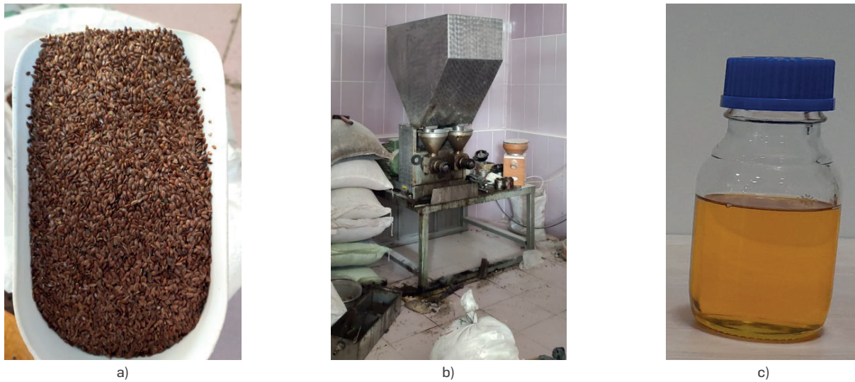
Figure 1. a) Linseed, b) Screw press, c) Linseed crude oil
