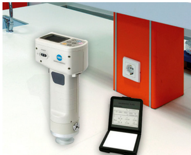
Figure 3. Minolta Chroma meter CR-400 used in the study.
