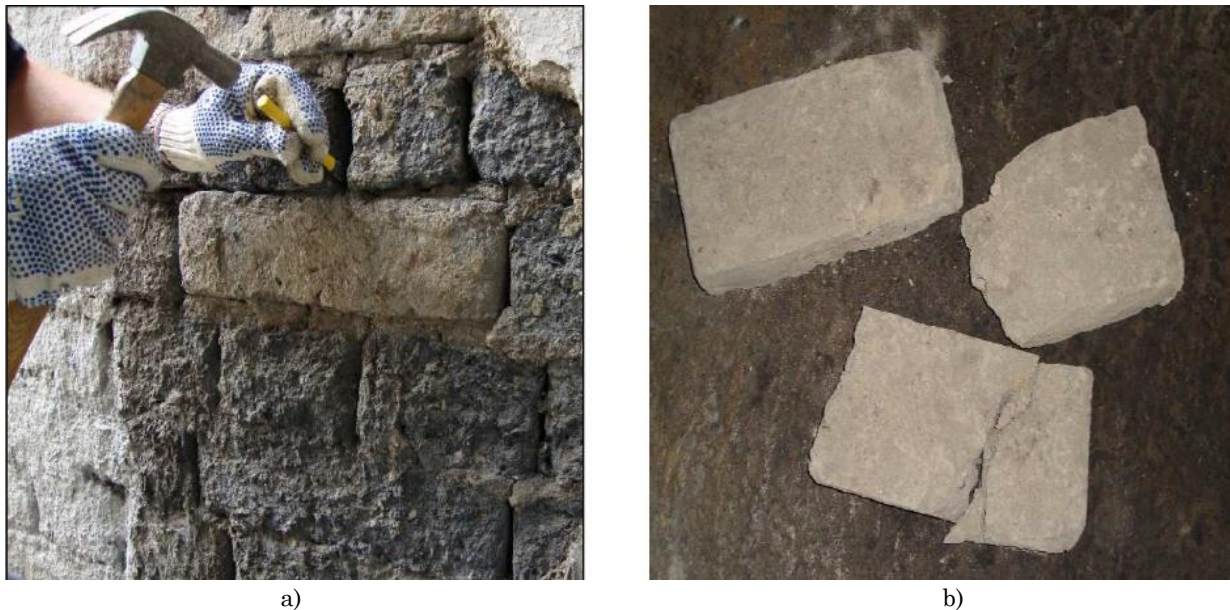
Figure 2. Samples of old adobe: a) recuperation of an adobe unit; b) recovered samples.
