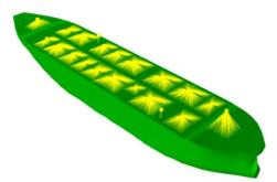
Figure 6. Mesh of the 3D hull model of the FPSO vessel, adding the masses of the equipment modules. This model is developed using Sesam GeniE software.
