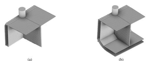
Figure 15. (a) Geometry A of the crane pedestal support frame that regards a part the main deck with the crane pedestal to the waterline; (b) Geometry B that comprises the full 3D model of the crane pedestal support frame.
