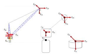
Figure 12. Free body diagram of the offshore crane that includes the force components on the work points of the crane, considering the crane pedestal.
