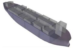
Figure 4. 3D hull model considering equipment modules of the FPSO vessel, which is obtained with Sesam GeniE software.
