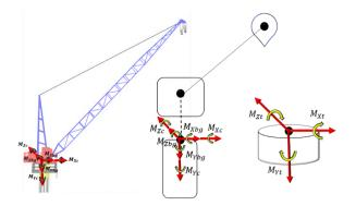
Figure 13. Free body diagram of the moment components on the offshore crane pedestal.
