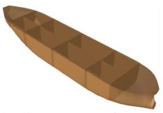
Figure 3. 3D hull model including different compartments of the FPSO vessel, which is generated with Sesam GeniE software.
