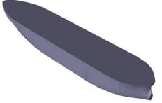
Figure 2. 3D hull model of the FPSO vessel, which is developed using Sesam GeniE software.
