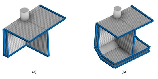
Figure. 17. Geometrical boundary conditions (fixed) in the edges of the 3D models of the crane pedestal support frame: (a) geometry A and (b) geometry B.
