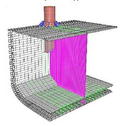
Figure 14. 3D model of the crane pedestal support frame used for the structural analysis of the main deck of the FPSO vessel. This model is done using Rhinoceros software.
