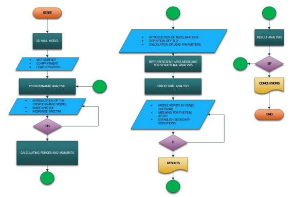
Figure 1. Flowchart of the stages of the methodology proposed for the structural analysis of a main deck of the FPSO vessel supporting an offshore crane.
