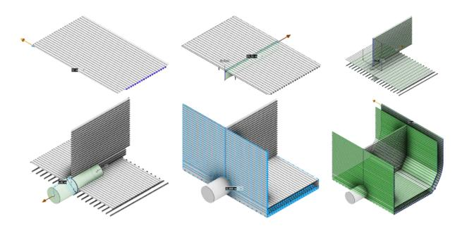
Figure 16. View of the different components of a 3D model of the crane pedestal support frame of the main deck of the FPSO vessel supporting an offshore crane. This 3D model was developed using Inventor software.
