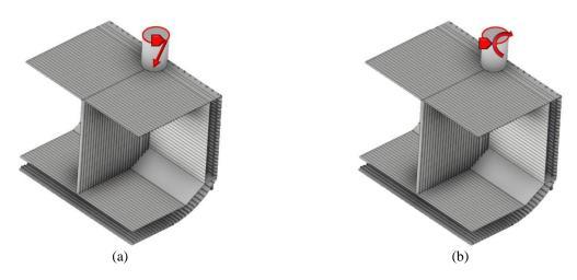
Figure 18. 3D model of the crane pedestal support frame of geometry B, including the maximum (a) force and (b) moment vectors.
