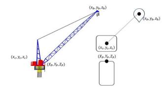
Figure 11. Schematic view of the three points of the offshore crane used to calculate the force and moment components.
