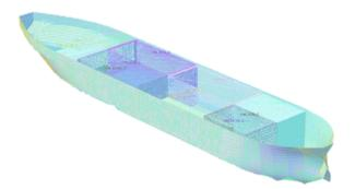
Figure 7. 3D hull model with equilibrium condition of the FPSO vessel, which is obtained using Sesam HydroD software.
