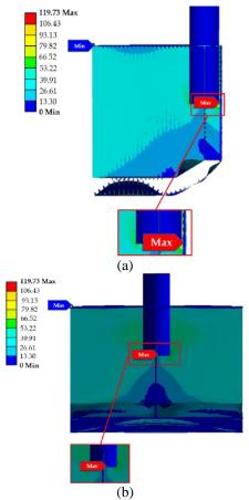
Figure 19. Distribution of von Mises stress of the FEM model of the crane pedestal support frame for the geometry A, considering the crane in bow section of the vessel and under regular operating conditions: (a) profile view and (b) side view.
