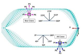
Figure 9. Five operating points of the offshore crane on both bow and alf sections of the FPSO vessel under operating conditions (calm sea).
