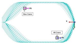
Figure 10. Operating points of the offshore crane on both bow and alf sections of the FPSO vessel under hurricane conditions.
