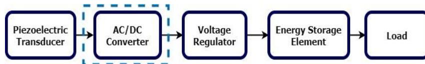
Figure 1. Schematic view of the main components of a typical piezoelectric energy harvester with AC/DC converter and storage system [9].
