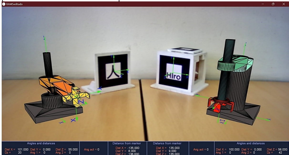
Figure 7. Program 2 "Serial Manipulators": The program prints the angles and distances of the joints from left to right and the separation between the end effector concerning the marker. The program presents the same data for the next manipulator.
