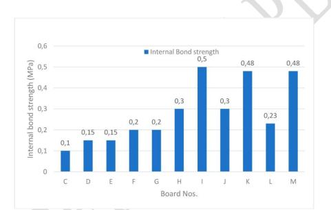
Figure 5: Internal bond strength of rice straw particles and wood fibers.
