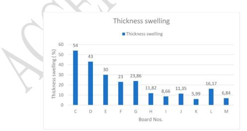
Figure 4: Thickness swelling properties of Rice straw particles and wood fibers,
