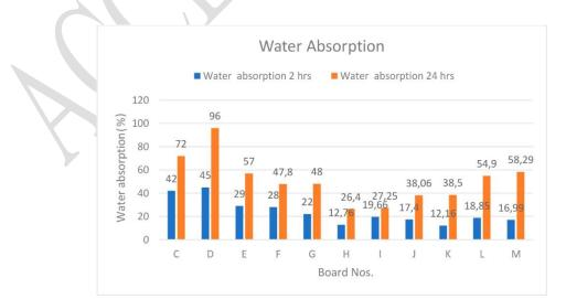
Figure 3: Water absorption properties of rice straw particles and wood fibers.
