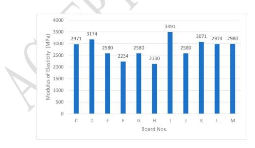
Figure 7: Modulus of elasticity of Rice straw particles and wood fibers.
