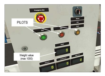
Figure 5. Detail of the layout's control panel
