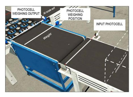
Figure 4. Detail of the conveyor belts and sensors in the layout
