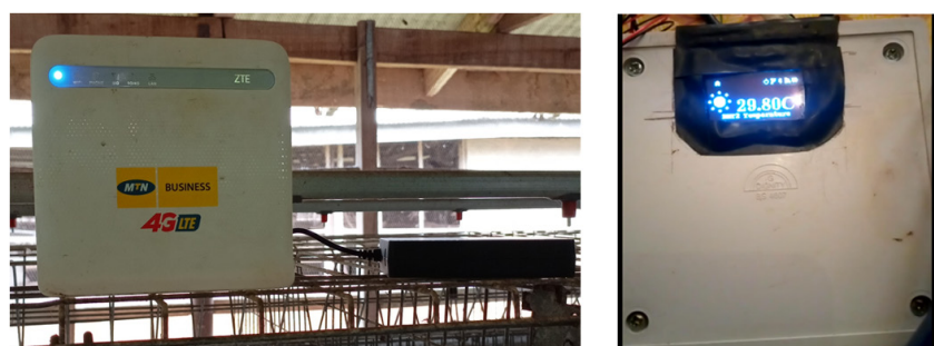
Figure 4. IoT-based sensors showing (a) a 4G LTE router and (b) a Sensor with an LCD.
