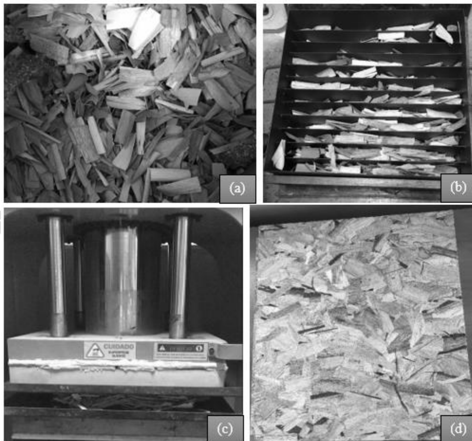
Figure 1: Production process: (a) Balsa wood chips; (b) particle forming and guiding mold; (c) Mattress pressing; (d) Balsa wood OSB panel.
