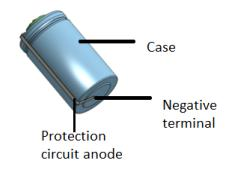
Figure 11. Cylindrical battery schematic. Source: Authors
