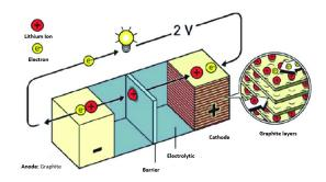
Figure 4. New composition of the Ion-Lithium battery. Source: Authors
