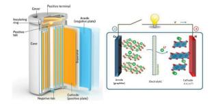
Figure 3. Parts that make up the Ion-Lithium battery. Source: (González, 2013).
