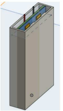
Figura 6. External battery configuration. Source: Authors
