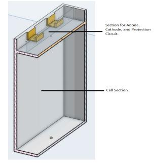
Figure 7. Internal battery configuration. Source: Authors
