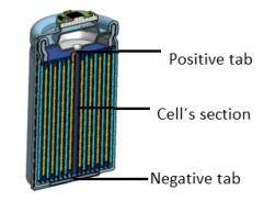
Figure 12. Internal schematic of the battery. Source: Authors
