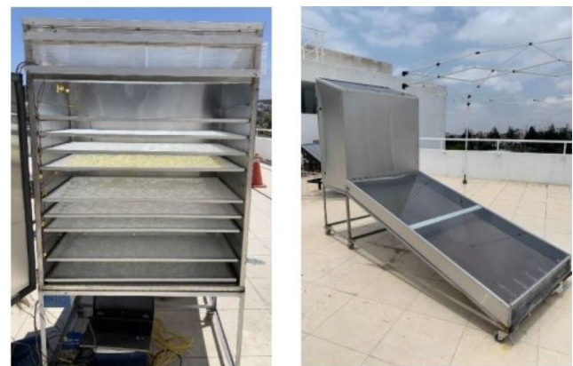
a) Front view b) Side view Figure 4. Mixed type active solar garlic dryer. Source: Own photograph.
