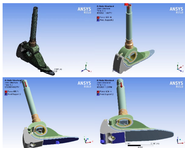
Figure 10. Static structural model with the three types of boundary conditions, i.e. the areas of fixation and the area of the applied load: (a) meshed process; (b) patient standing; (b) beginning of the walking cycle; (c) end of the walking cycle
