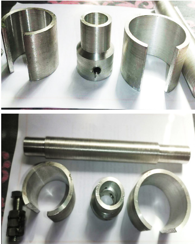
Figure 6. The fabricated prosthesis limb parts were processed in the turning machine Source: Authors
