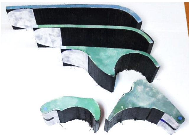
Figure 7. Cutting the parts of the artificial foot using a band saw machine Source: Authors
