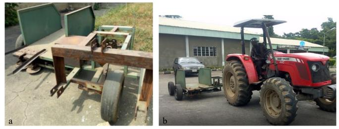
Figure 1. The fabricated kenaf harvester: (a) front view of the fabricated kenaf harvester; (b) the developed kenaf harvester mounted on a tractor.
