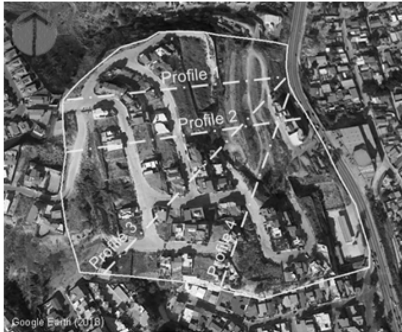
Figure 6. Profiles used for slope stability analysis.
