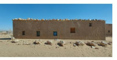
Figure 16: Facade of a housing unit in the *wilāyah* of Smara. Openings at different heights, reflecting the use of interiors and facilitating cross-ventilation (2022)
