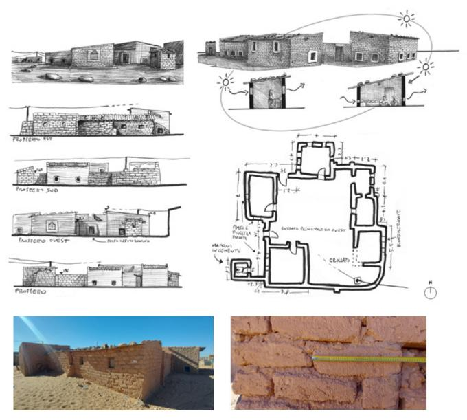
Figure 15: Drawings and architectural surveys of a housing unit in the *dā 'ira* of Bir Lehlu, *wilāyah* of Smara. Windows are positioned according to room function, favoring cross-ventilation. Adobe walls offer good thermal insulation (2022)
