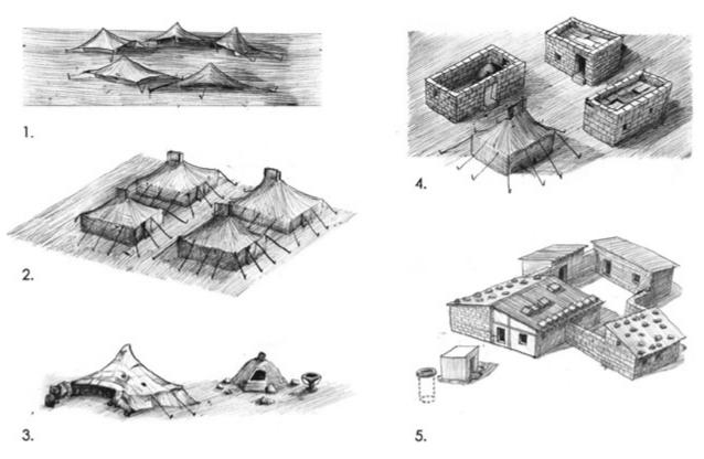
Figure 8: Five stages of camp evolution: 1. The early camps were made by arranging tents in the circular *anawāl* form. 2. Checkerboard arrangement of new tents provided by international organizations. 3. Reorganization of spaces and erection of an earthen oven. 4. Construction of the first adobe buildings with fabric roofs. 5. Finally after the 2015 flood, concrete houses
