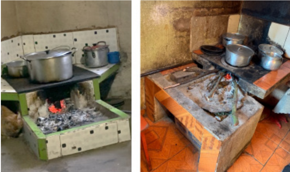
Figure 3. Stoves rebuilt with ICS parts
