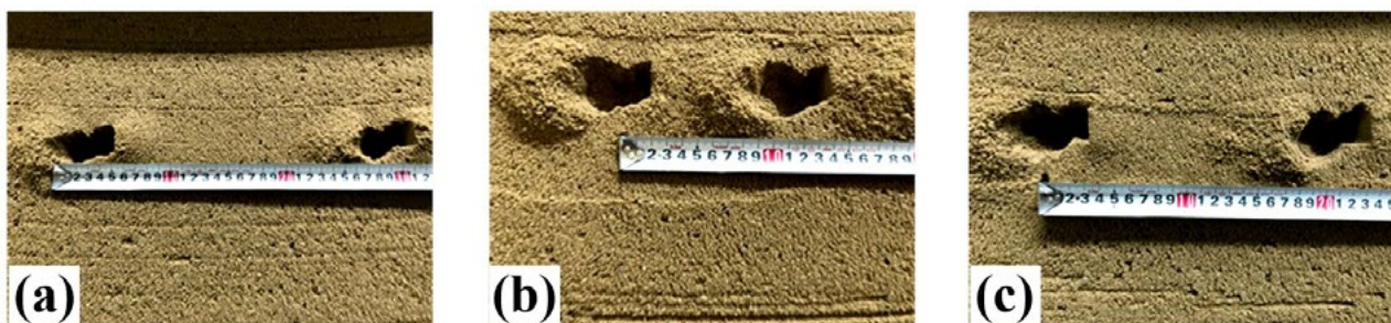
Figure 9. Planting interval for the rotary planting mechanism determined using (a) 0.10, (b) 0.15, and (c) 0.20 m s -1 forward speeds at 60 rpm.
