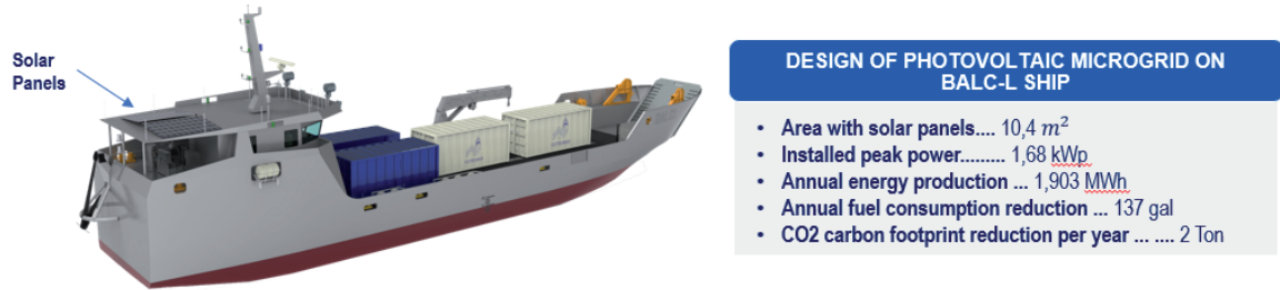
Fig. 7. BALCL design with implementation of solar panels.
