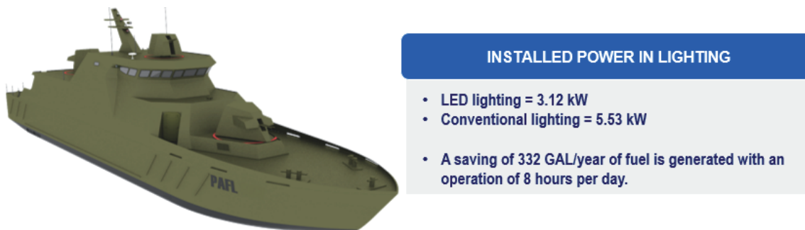
Fig. 6. Implementation of LED lighting in PAF-L.
