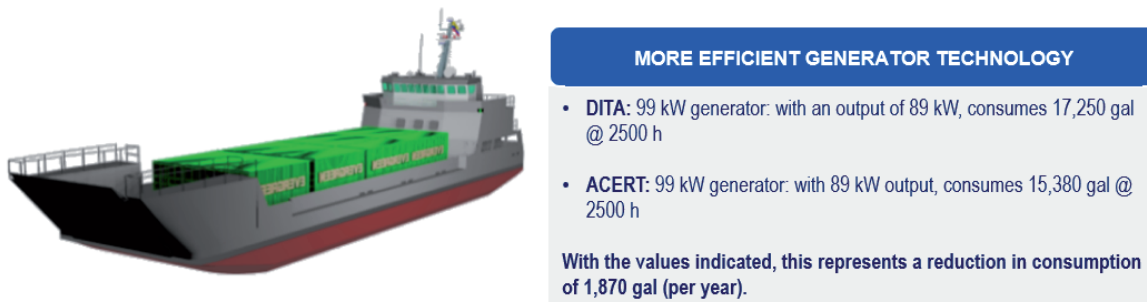
Fig. 5. ACERT (Advanced Combustion Emission Reduction Technology) Genset in BDA.
