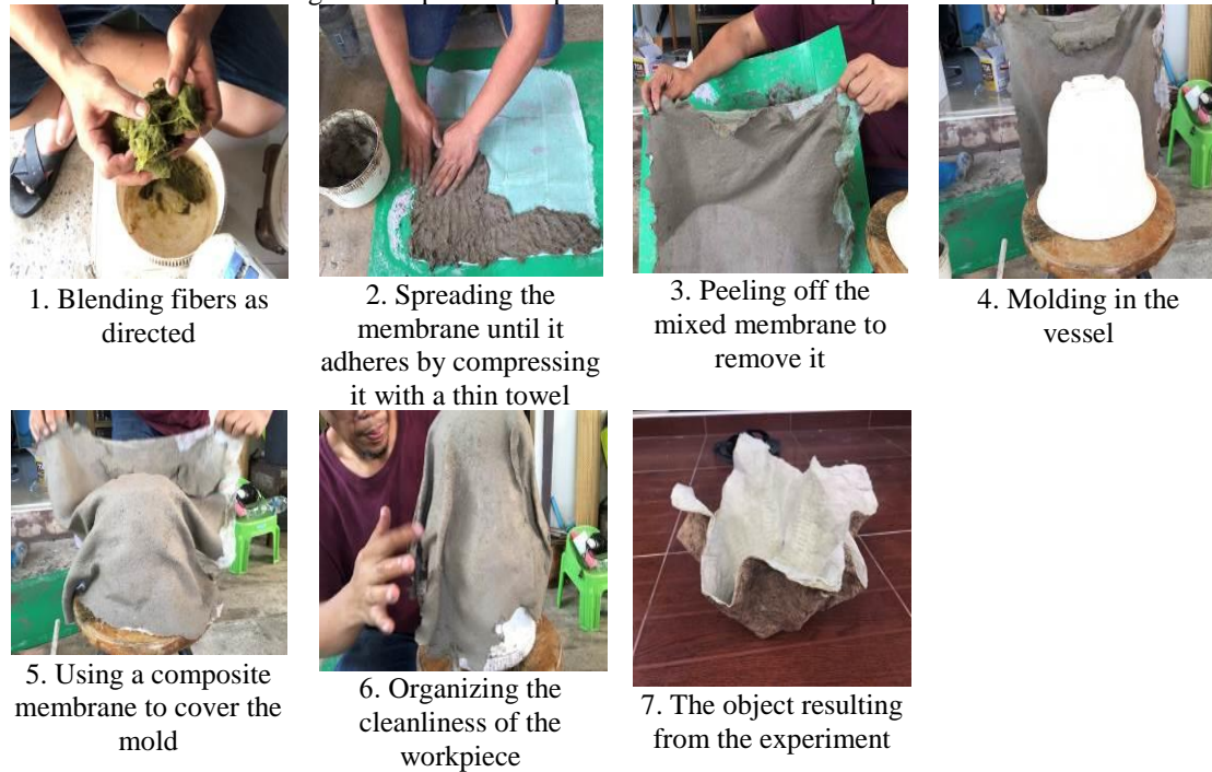
Figure 8 Experimental process for material development
