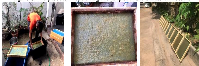
Figure 6 The process of spooning the pulp to make sheets of material
