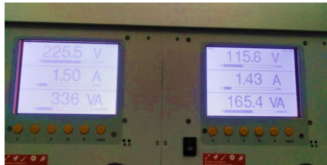
Figure 30. Power input and output measured data result. Source: The author.
