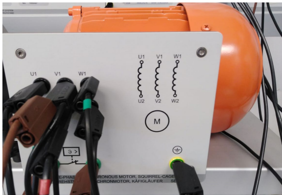
Figure 13. Three phase induction machine of Training systems for electric machines, drivers and power electronics. Source: The author.
