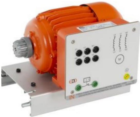
Figure 12. Three phase induction machine of Training systems for electric machines, drivers and power electronics. Source: The author.
