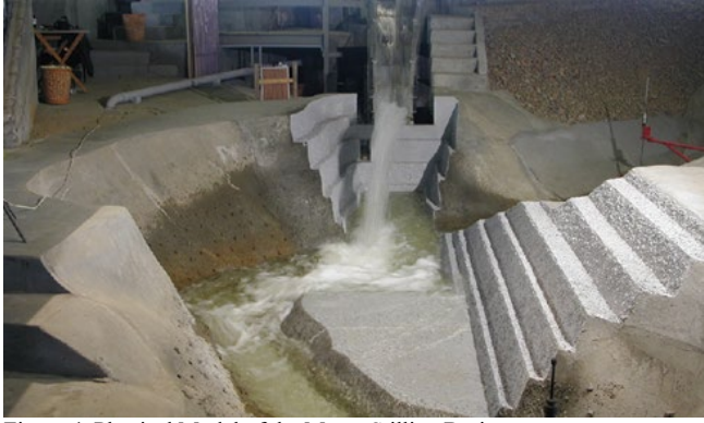
Figure 4. Physical Model of the Mazar Stilling Basin. Source: Own elaboration.
