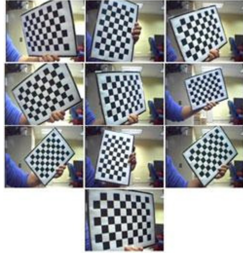
Fig. 5. Self-collection data from MVLab used to obtain the intrinsic and extrinsic values.
