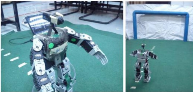
Fig. 11. Wireless camera attached to a robot for the distance estimation test.
