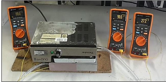
Figure 11. Tests performed with a constant 1000-watt heat source. Source: Own elaboration
