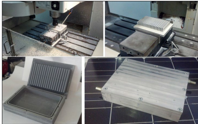
Figure 7. Simulation and calibration, coordinate system adjustment, planned, grinding, fin machining, machined and assembly. Source: Own elaboration.
