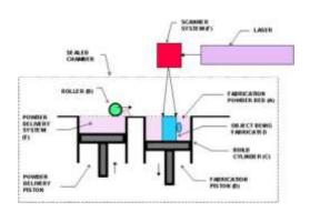
Figure 8: Selective Laser Sintering (SLS)
