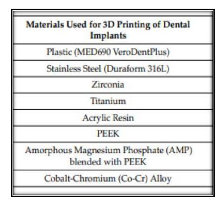
Figure 16: Materials used 3D printed dental implants
