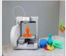
Figure 6: Fused deposition modelling (FDM)
