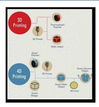
Fig 17: Illustration outlining the difference between 3D and 4D printing
