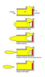
Figure 9: Thermal Inkjet Printing (TIJ)
