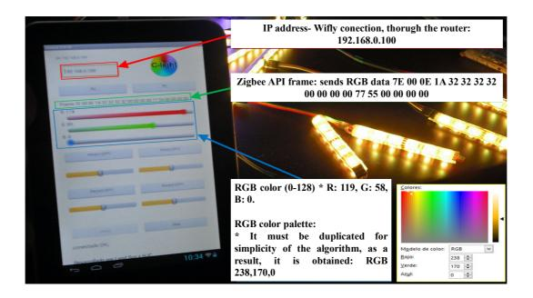
Fig. 9. APP Mobile cellular Control Wireless Network. Source: the authors.
