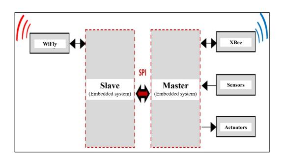
Fig. 2. Master-slave ZigBee & Wi-Fi interconnectivity. Source: Own elaboration.
