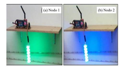
Fig. 5. ZigBee communication card with power module and RGB LED control. (a) Node 1 (RGB in green), (b) Node 2 (RGB in blue). Source: Authors.
