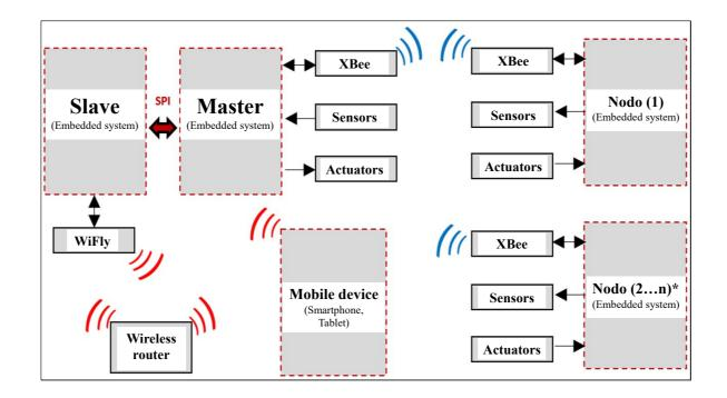
Fig. 3. ZigBee (blue) and Wi-Fi (red) interconnected networks structure. \*n: number of nodes (up to 64000 nodes). Source: Own elaboration.
