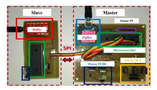
Fig. 1. ZigBee – Wifly Embedded System. Interconnectivity node. Source: The authors.
