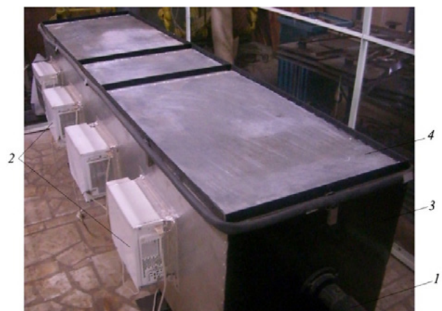
Figure 4. General view of the microwave dryer: 1, a shaft that provides rotation of a timber pile; 2, magnetrons; 3, the housing of the microwave dryer; 4, a cover of the working chamber made of steel mesh.
